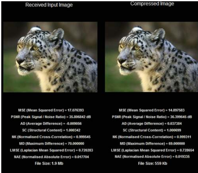
Fig. 5: Comparison of the image properties of the input image and that of output image when processed through the presented region-specific wavelet compression algorithm
