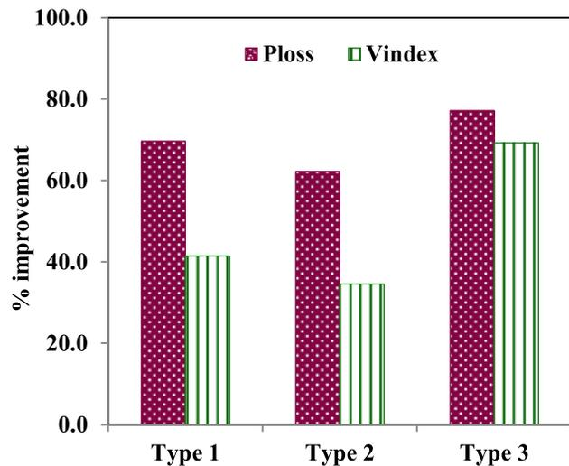
FIG. 8. Percentage improvement in real power loss and voltage deviation for residential load.
