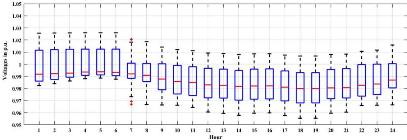
FIG. 12. Hourly box plot of voltage for a day-mixed load.
