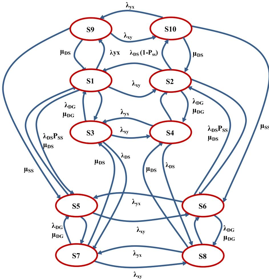
FIG. 1. Markov model for the distribution system.
