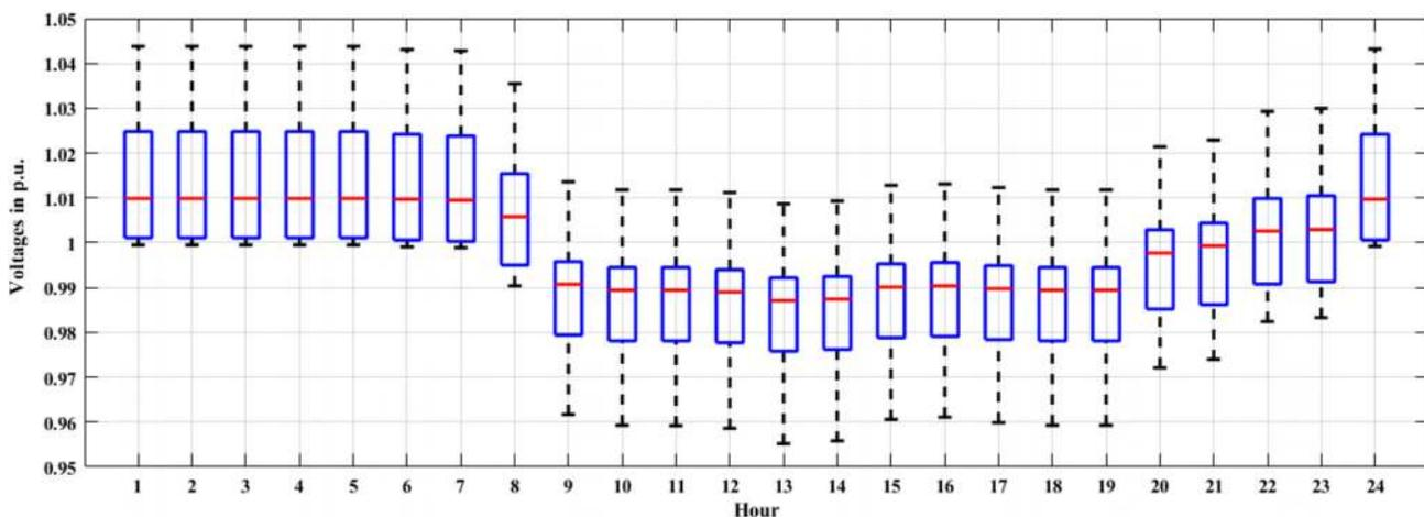
FIG. 9. Hourly box plot of voltage for a day-commercial load.
