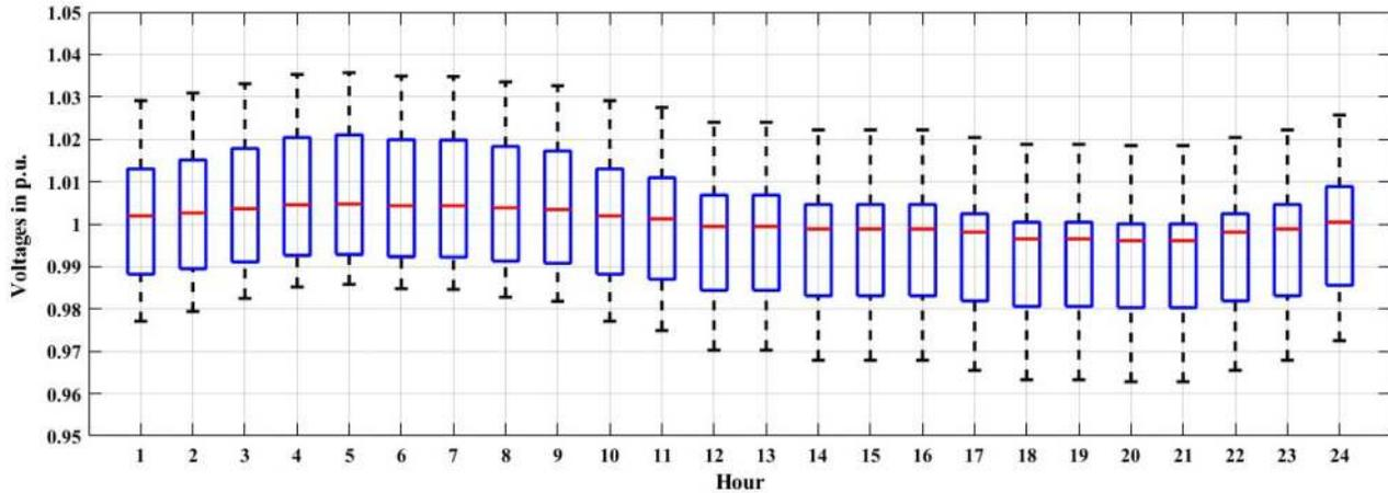
FIG. 6. Hourly box plot of voltage for a day-residential load.
