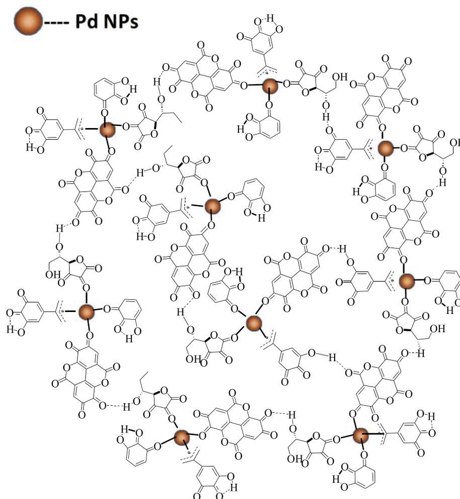
**Fig. 3** Schematic representation of phytochemicals based stabilization of Pd NPs.
