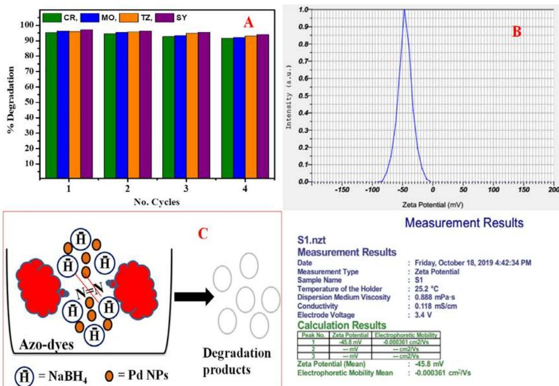
**Fig. 9** The catalytic efficiency of Pd NPs for reduction of CR, MO, TZ and SY (A), Zeta potential analysis of Pd NPs collected after reduction by DLS study (B) and Possible mechanism of azo dye reduction by NaBH<sub>4</sub> as reducing agent and Pd NPs as catalyst (C).
