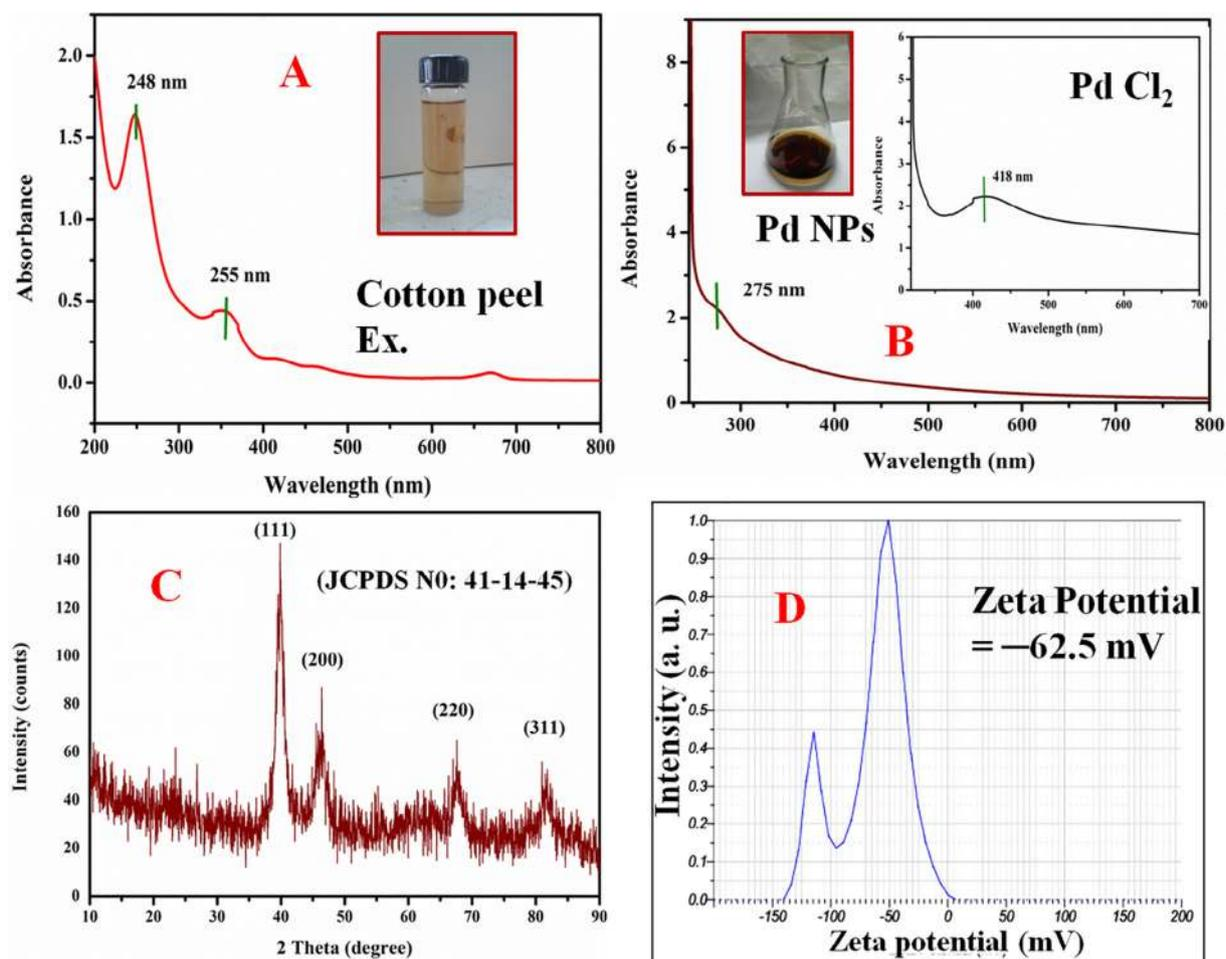
**Fig. 1** UV-Vis spectra of cotton peels extracts (A), synthesized Pd NPs using aqueous cotton peels extracts (inset UV-Vis spectrum of Pd chloride solution (B), XRD pattern of synthesized Pd NPs (C) and zeta potential of Pd NPs aqueous dispersion by DLS analysis (D).
