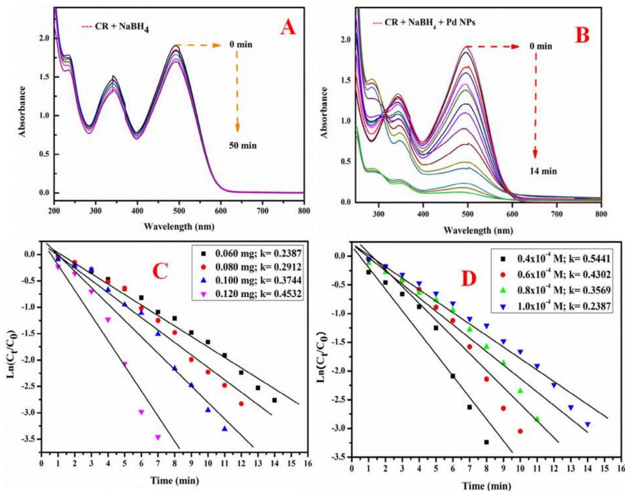
**Fig. 5** UV-Vis absorption spectra for the reduction of Congo Red dye by  $\text{NaBH}_4$  aqueous solution without catalyst Pd NPs (A), with catalyst Pd NPs (B), Effect of Pd NPs doses (mg) on the reduction kinetics of Congo Red dye (C) and Effect of Congo Red dye concentration (M) on reduction kinetics of Congo Red dye at constant dose of catalyst Pd NPs (D).
