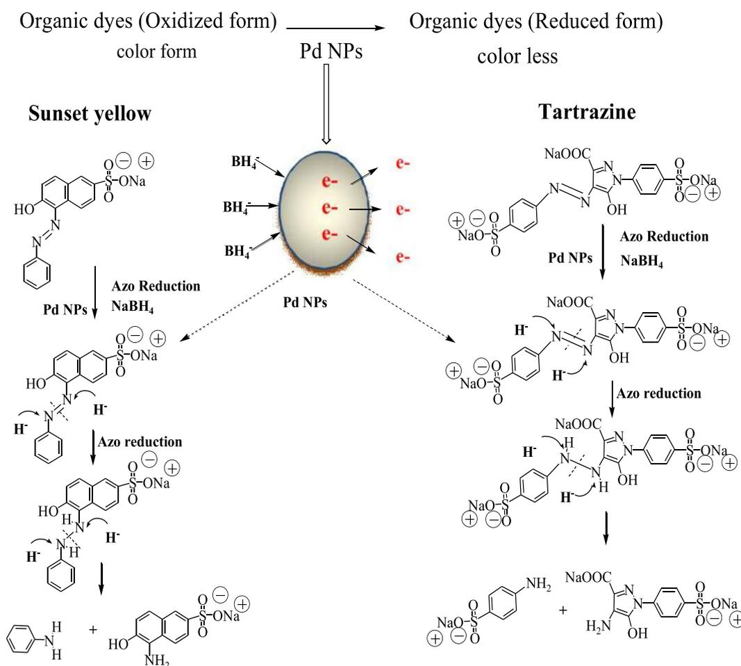
**Fig. 7** Plausible mechanism for the reduction of Sunset Yellow and Tartrazine dyes by NaBH<sub>4</sub> aqueous solution with catalyst Pd NPs.
