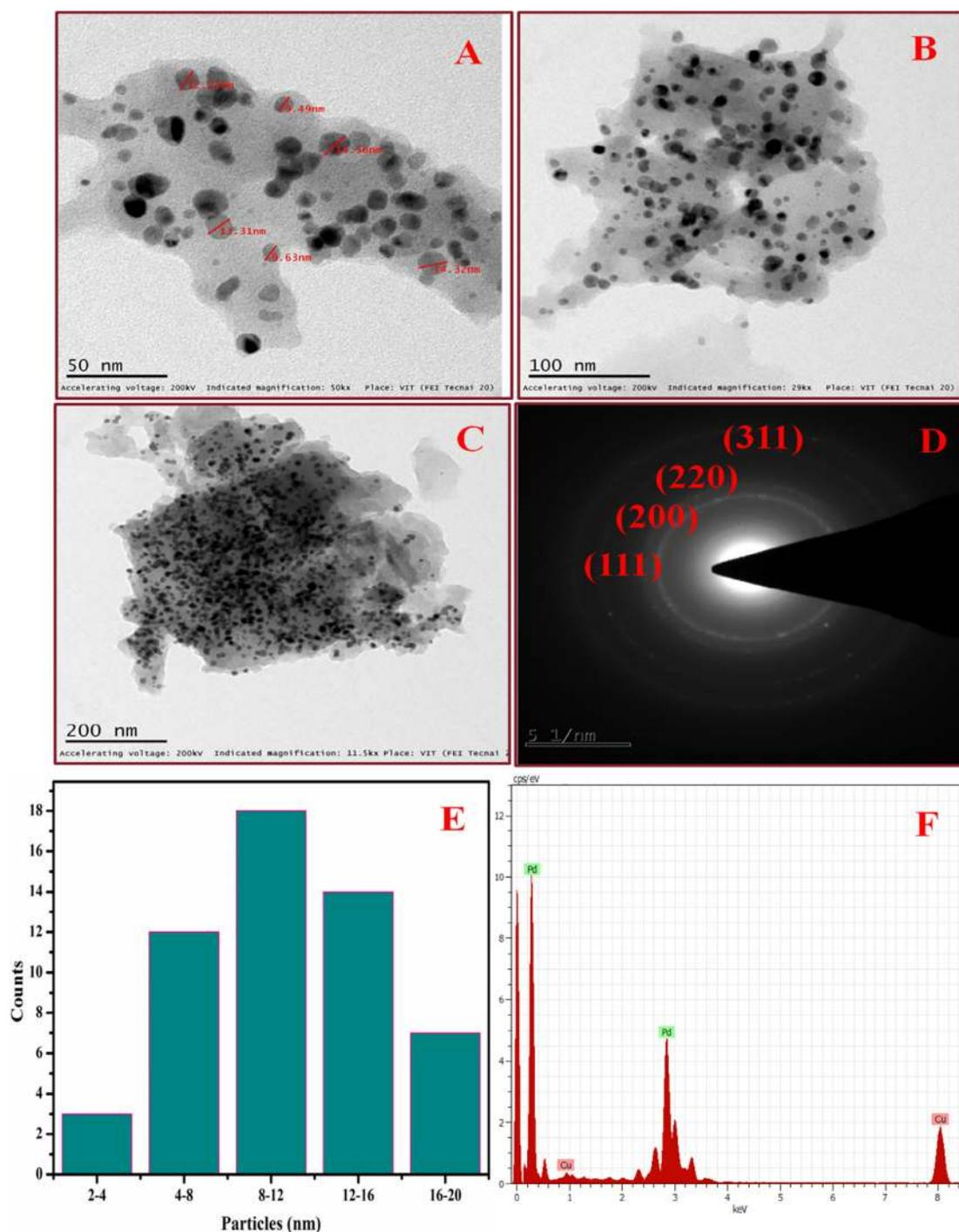
**Fig. 4** TEM images of synthesized Pd NPs at different magnification 50 nm (A), 100 nm (B), 200 nm (C), SAED pattern of Pd NPs (D), Particles size distribution of Pd NPs (E) and EDX spectrum of Pd NPs (F).
