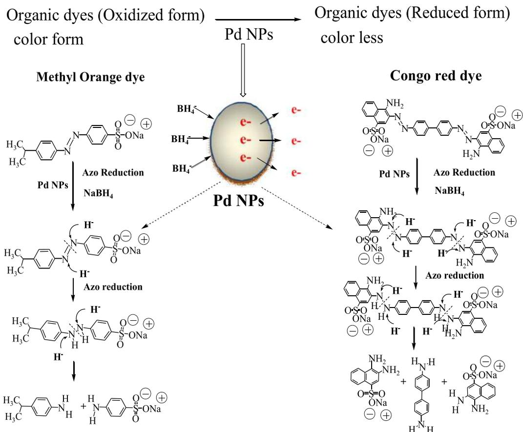
**Fig. 8** Plausible mechanism for the reduction of Methyl Orange and Congo Red by NaBH<sub>4</sub> aqueous solution with Pd NPs as catalyst.
