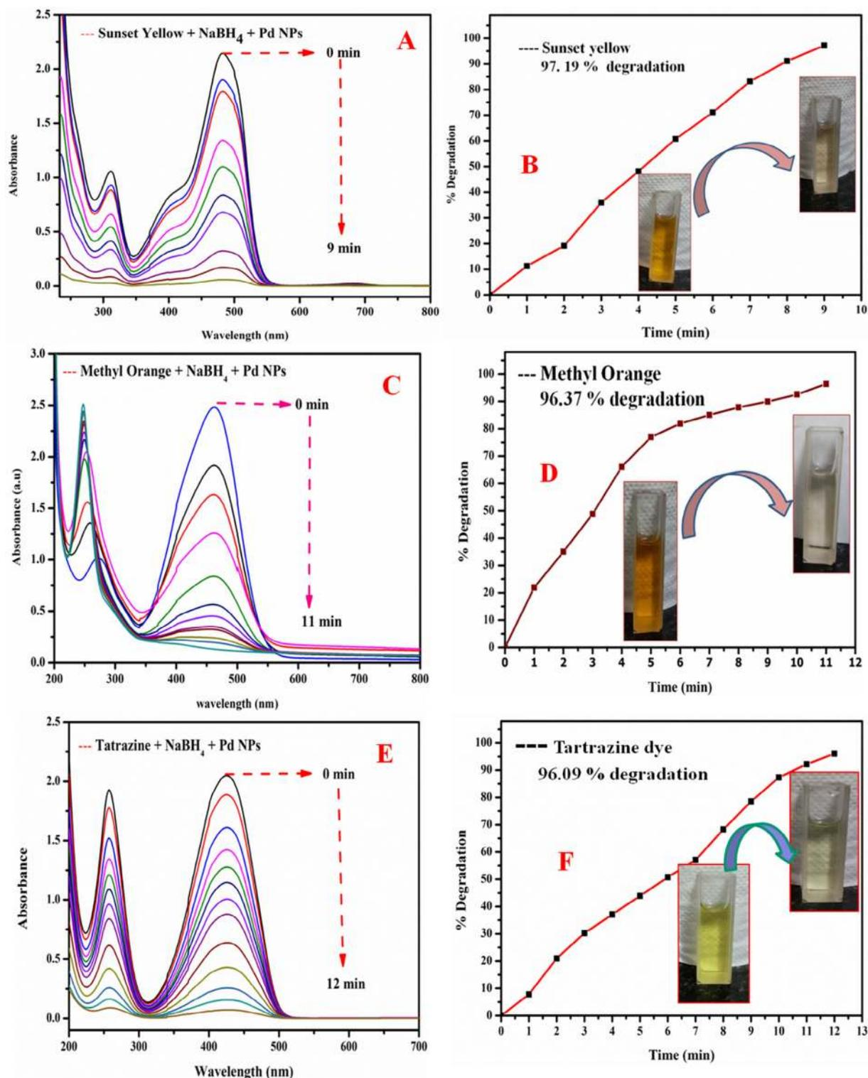
**Fig. 6** Reduction of Sunset Yellow (SY) (A), Methyl Orange (MO) (C), Tartrazine (TZ) (E) by  $\text{NaBH}_4$  aqueous solution with catalyst Pd NPs and degradation kinetics of SY (%) (B), MO (%) (D) and TZ (%) (F) with time by  $\text{NaBH}_4$  aqueous solution with catalyst Pd NPs.
