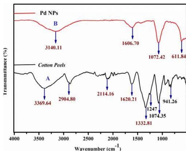
**Fig. 2** FT-IR spectra of cotton peels (A) and synthesized Pd NPs using cotton peels aqueous extracts (B).
