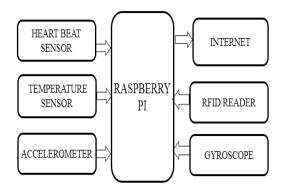
Figure 1. Block diagram.
