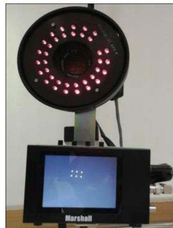
Figure 1: Camera system with infrared illuminator (wall-mounted) and display unit. Marker dots are seen in the monitor
