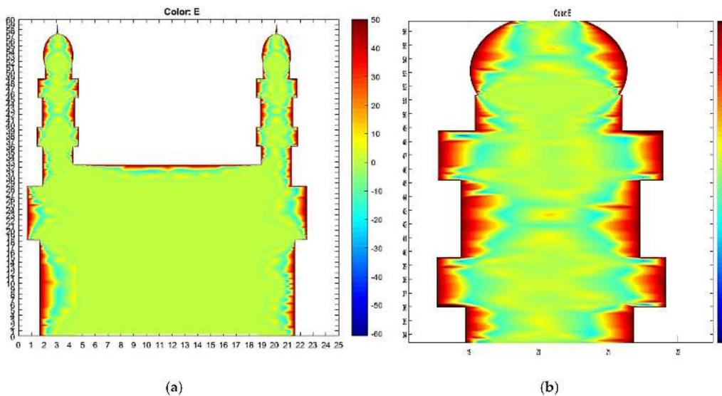
**Figure 15.** (a) Plot of simulation for obtaining skin depth with  $\sigma = 0.02$  at a frequency of 10 kHz; (b) detailed view of skin depth and depth of penetration at vulnerable points of the structure.
