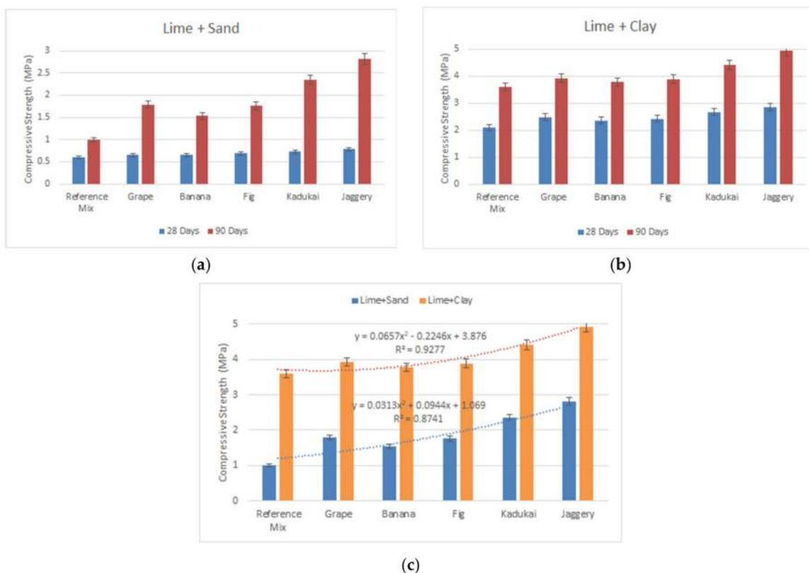
**Figure 7.** Compressive strength: (a) 28 and 90 curing days for lime–sand mixtures, (b) 28 and 90 curing days for lime–clay mixtures, (c) comparison between lime–sand and lime–clay mixtures at 90 curing days. Error bars indicate standard deviation. A multiple regression model was formulated using the compressive strength values; R2 values of 0.927 for lime–clay and 0.874 for lime–sand mixes were obtained, which established an excellent accuracy of the experimental values [56].
