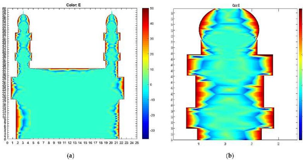
**Figure 14.** (a) Plot of simulation for obtaining skin depth with  $\sigma = 0.02$  at a frequency of 250 kHz; (b) detailed view of skin depth and depth of penetration at vulnerable points of the structure.
