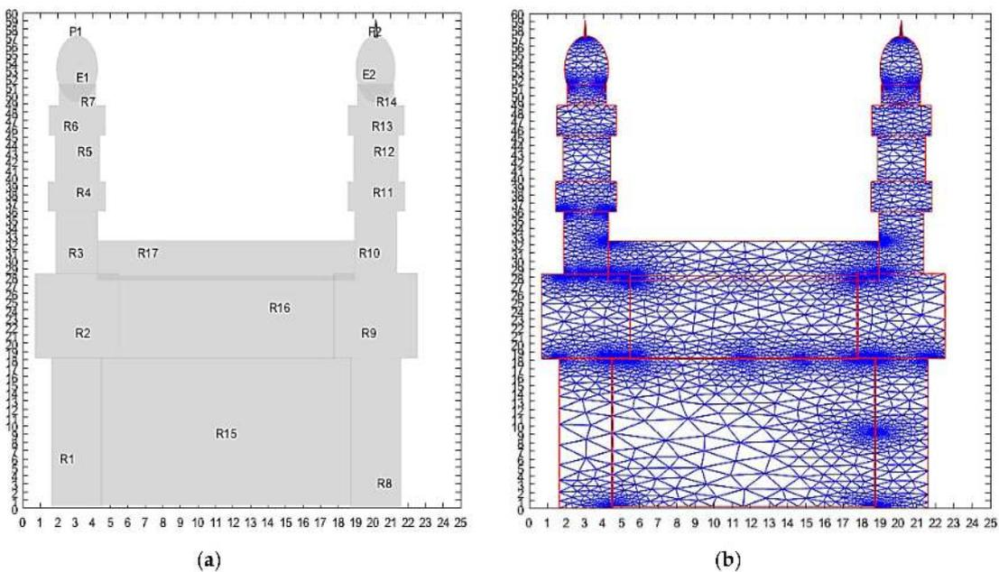
**Figure 13.** (a) Layout of the Charminar Monument for simulation of the role of electrical conductivity and skin depth; (b) simulation of Finite Element Method (FEM)-based solution of the heritage structure.
