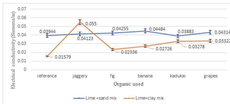
Figure 9. Electrical conductance for lime–sand and lime–clay mixtures.
