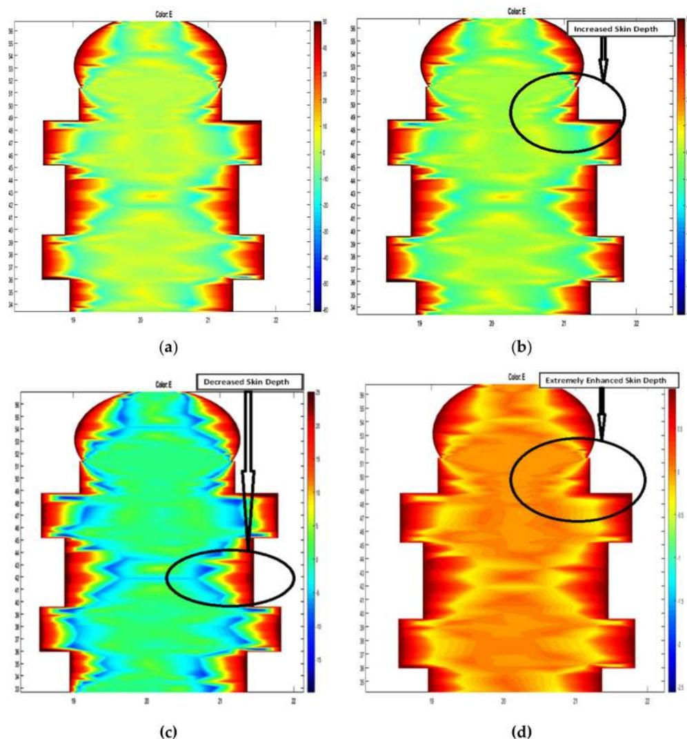
**Figure 16.** Comparison for depth of penetration at 10 kHz for varying lime mortar mixes: (a) reference mix (lime–clay), (b) lime mortar of the heritage monument (from Charminar), (c) lime-clay + kadukai, and (d) cement concrete mix. In (a–c) dielectric permittivity ( $\epsilon_r$ ) = 7 and magnetic permeability ( $\mu_r$ ) = 1–3; in (d) dielectric permittivity ( $\epsilon_r$ ) = 12–29 and magnetic permeability ( $\mu_r$ ) = 1.
