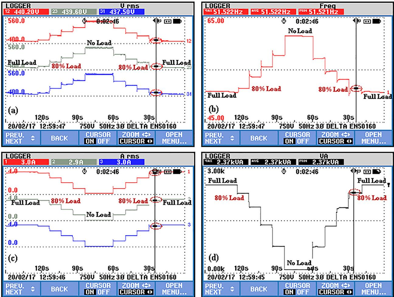
Fig. 4. Variation of output electrical quantities during load variation without regulation. (a) Voltage; (b) Frequency; (c) Current; (d) Power.
