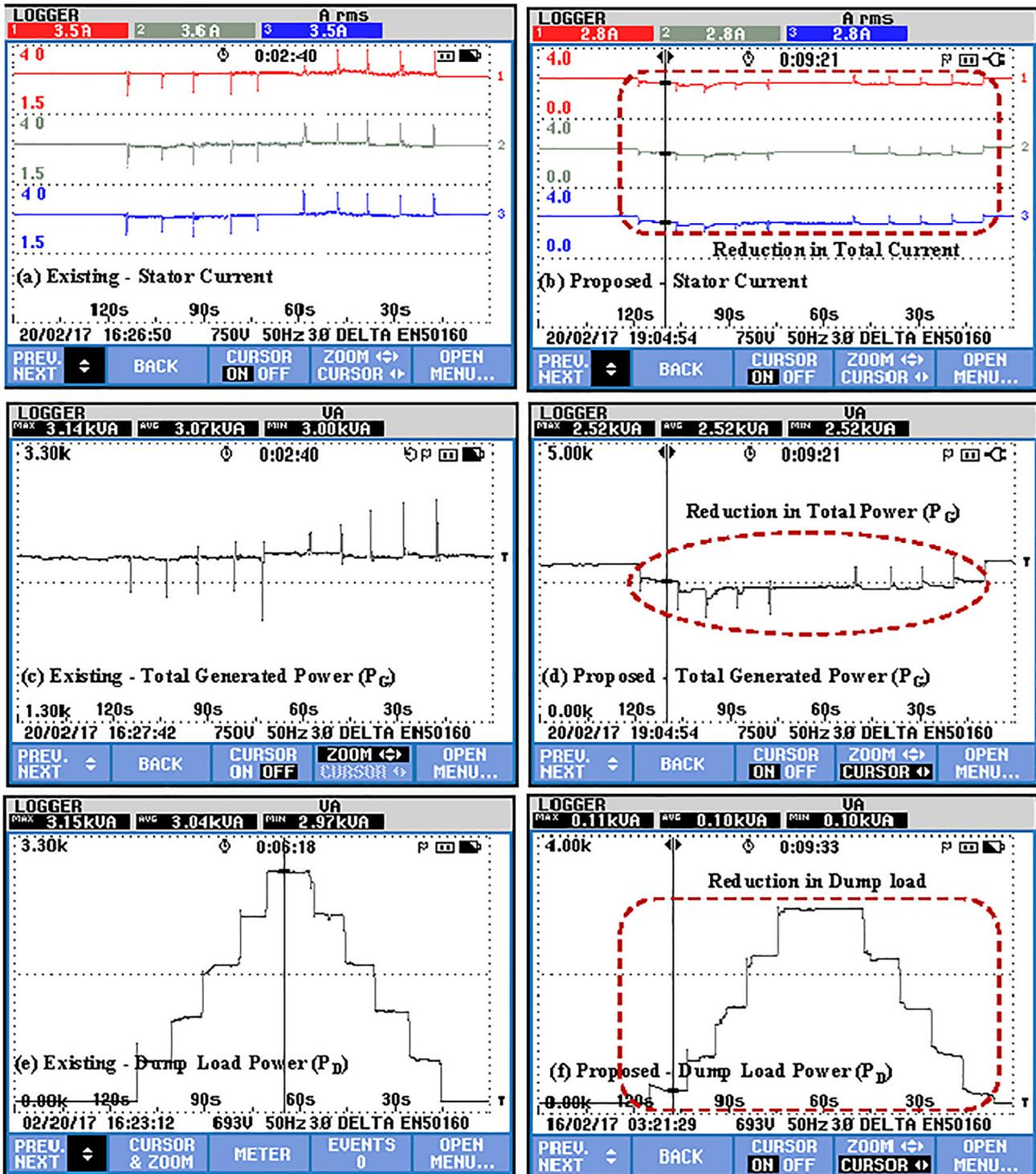
Fig. 12. Output electrical parameter of generator between existing and proposed strategy Existing - (a) Current; (b) Main Load power; (c) Dump load power Proposed - (b) Current; (d) Main Load power; (f) Dump load power.
