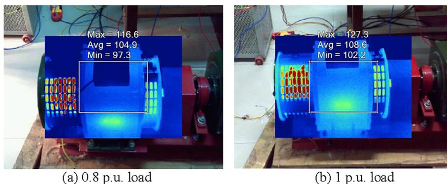
**Fig. 6.** Temperature variation under reduced dump load and full dump load in °F.
