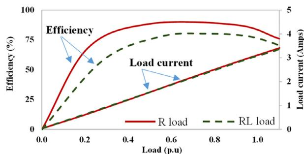
Fig. 3. Efficiency and current profile of synchronous generator.
