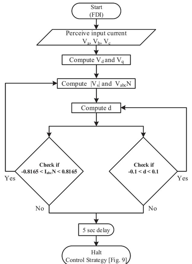
Fig. 7. Flow diagram for sensor fault detection and isolation.
