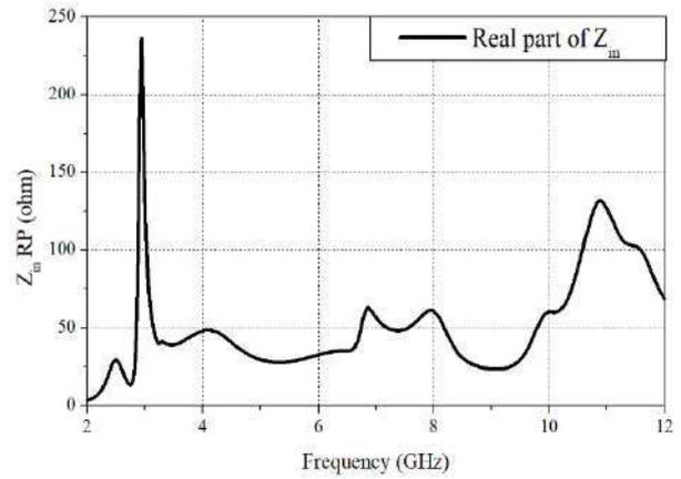
Fig. 21 Input impedance (Real part) of the antenna
