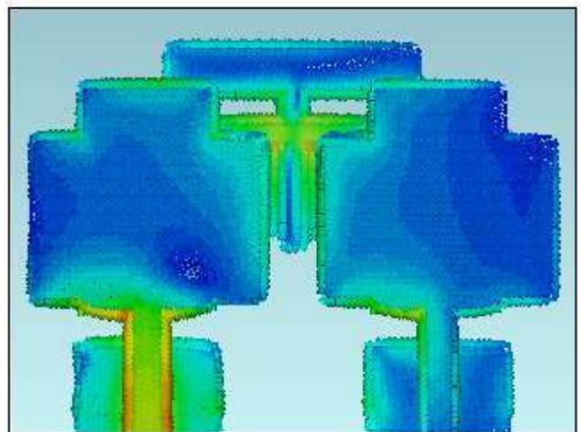
Fig.18 Surface current distribution of the antenna
