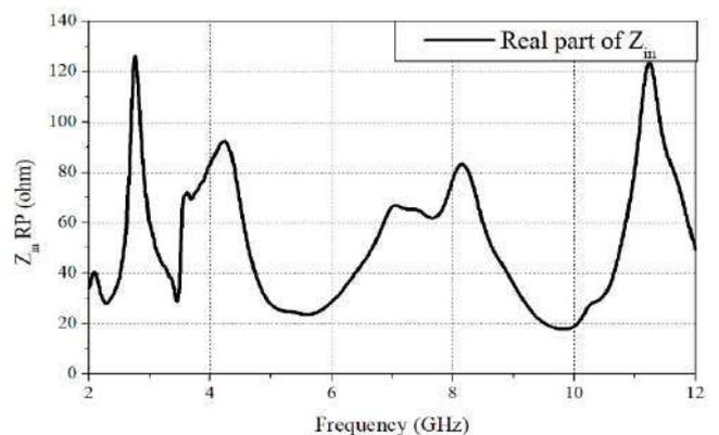
Fig.33 Input impedance (Real part) of the antenna
