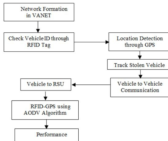
Figure 1. Framework for RFID-GPS using AODV in VANET
