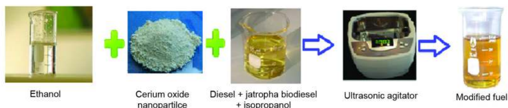
Figure 2. Schematic diagram of the modified fuel prepared by the two-step method
