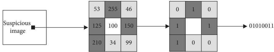
FIGURE 3: An example of a basic LBP operator.
