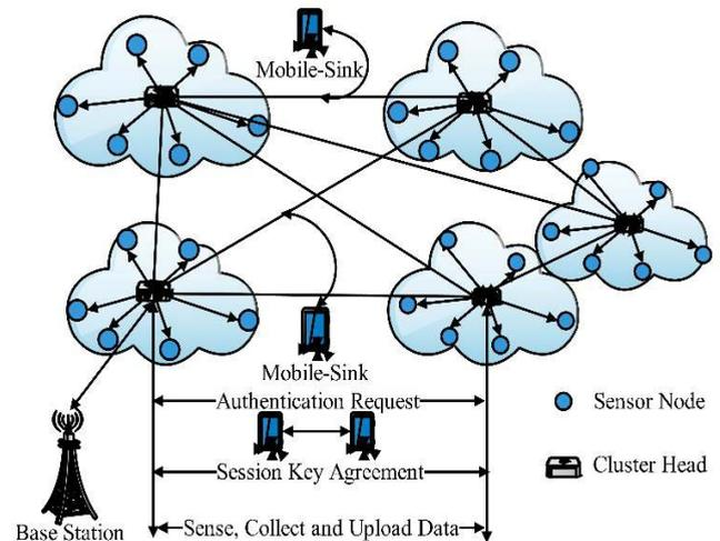
**FIGURE 1. Architecture of hierarchical Cloud Based WSNs.**
