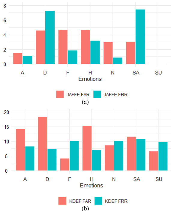
FIGURE 9. Plot of FAR and FRR metrics provided by testing (a) JAFFE and (b) KDEF databases for MLPNN with FV_{int\_norm\_1} . A - Angry, D - Disgust, F - Fear, H - Happy, N - Neutral, SA - Sad, SU - Surprise.
