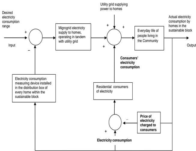
**Fig.3.** Flow diagram depicting the drivers of homeostatic control strategies to ensure efficient electricity supply and demand equilibrium based on energy and power consumption ranges per home consumers [10]. Source: owned elaboration.
