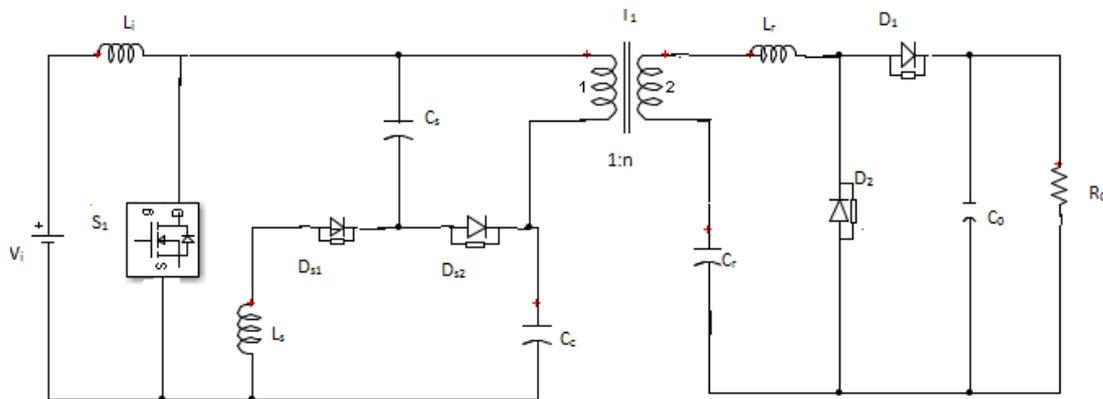
**Figure 1.** Proposed ZCS-ZVS Converter
