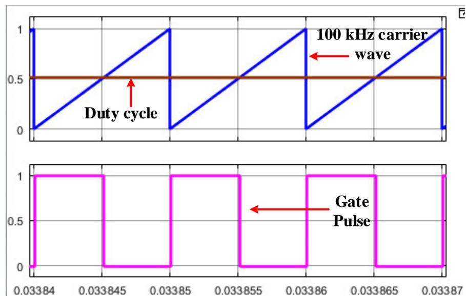
**Figure 5.** Simulation results of carrier wave, duty cycle and gate pulse
