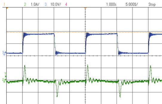
**Figure 9(a).** Hardware results of  $V_{GS}$  and  $I_D$
