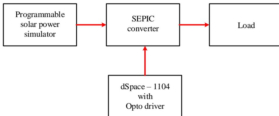
**Figure 4.** Block Diagram for propose system
