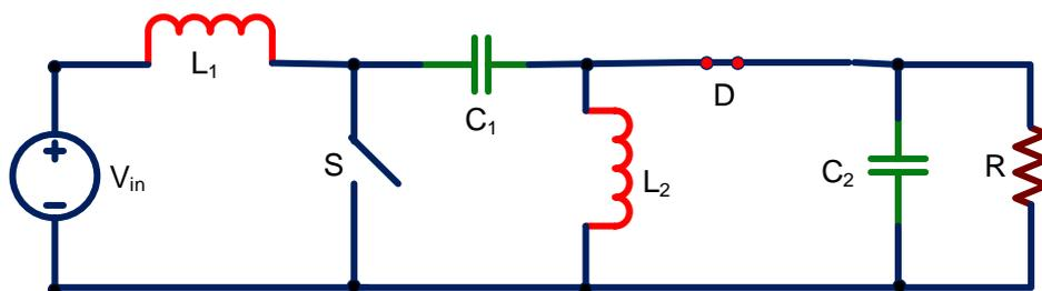
Figure 3. Circuit diagram for Switch S is closed
