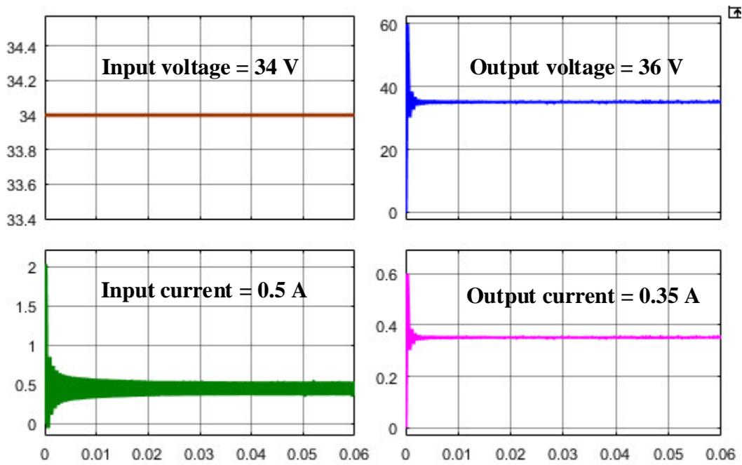
**Figure 6.** Simulation results of  $V_{in}$ ,  $I_{in}$ ,  $V_{out}$ , and  $I_{out}$
