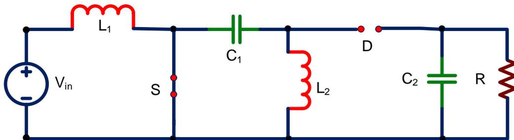
Figure 2. Circuit diagram for Switch S is closed
