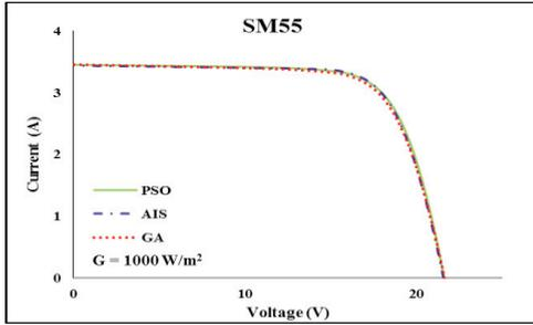
Fig. 1. Simulated I-V Curves for Different Optimisation Techniques
