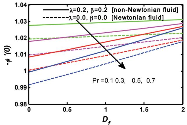
Fig. 15 Effect of  $Pr$  on  $-\phi'(0)$  against  $D_f$
