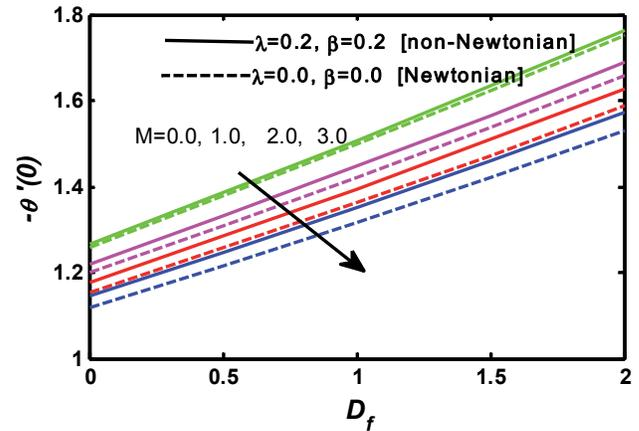
Fig.14 Effect of  $M$  on  $-\theta'(0)$  against  $D_f$
