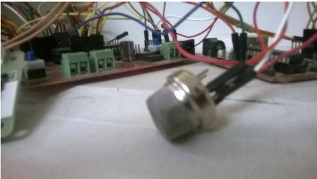
Figure 5. Interfacing MQ4 with AVR.
