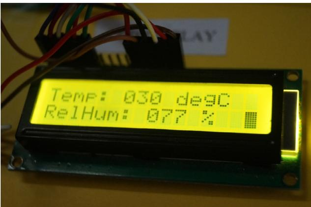
Figure 6. Interfacing LCD Display with AVR.
