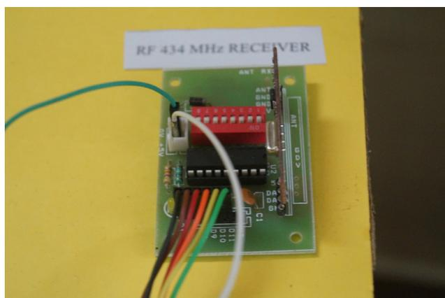
Figure 10. RF 434 MHz Receiver.
