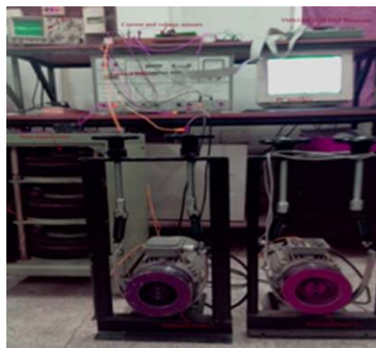
Fig. 5. Experimental set up of parallel-connected induction motor drive controlled by DSP TMS320F2812.
