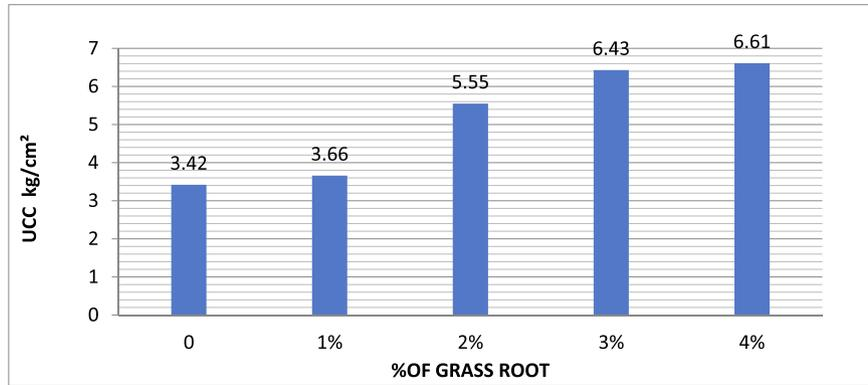
Fig. 8. The effect of UCC with the addition of various percentage of fibers.
