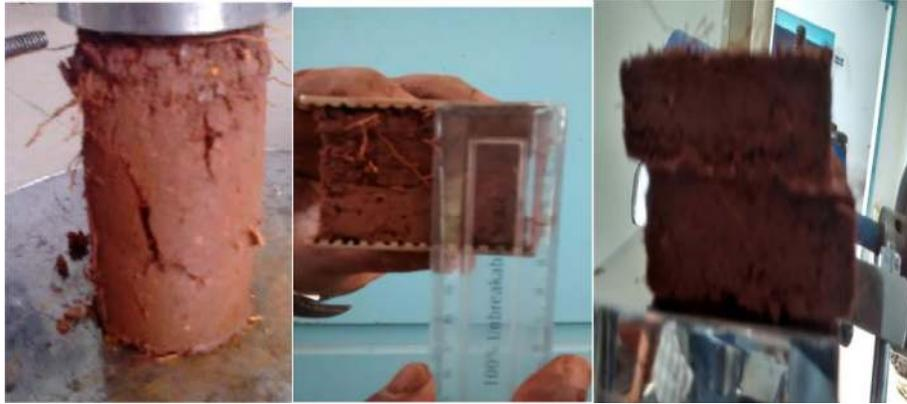
Fig. 5. Sample preparation for strength tests.
