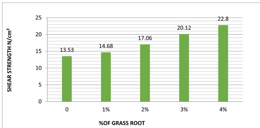
Fig. 7. The effect of Shear strength with the addition of various percentage of fibers.
