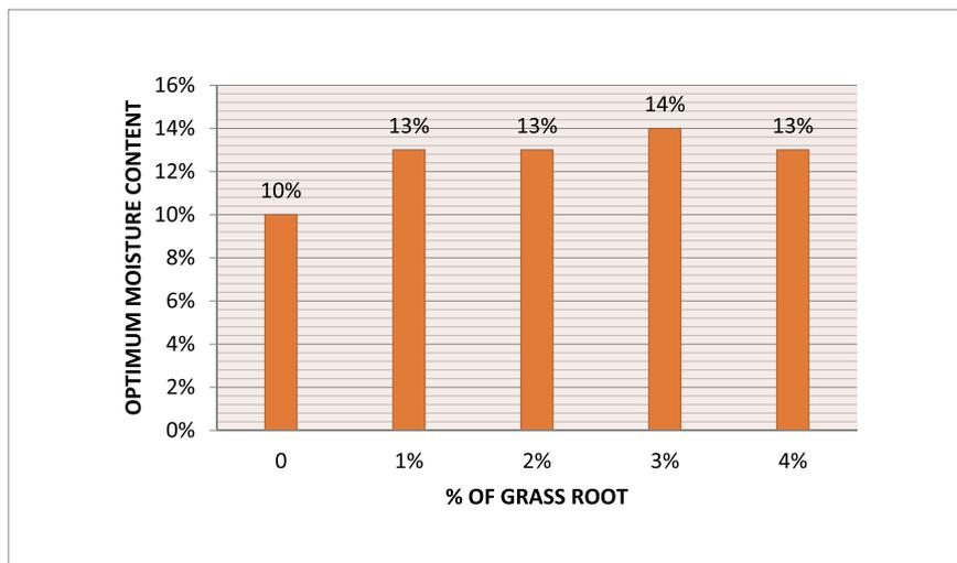
Fig. 6. The effect of OMC with the addition of various percentage of fibers.
