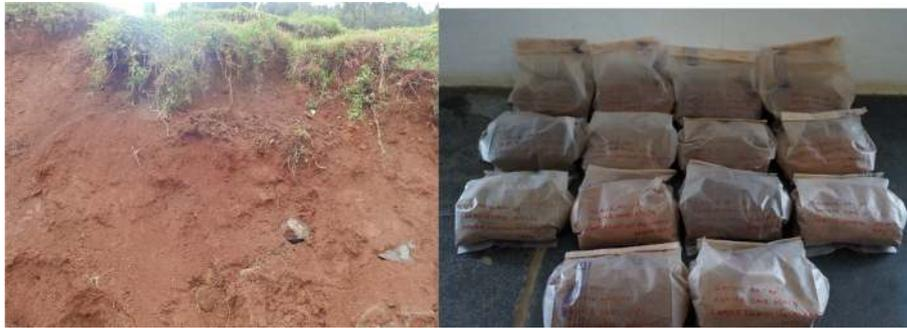
Fig. 1. a) Slope failed area from where soil is collected b) Soil samples.
