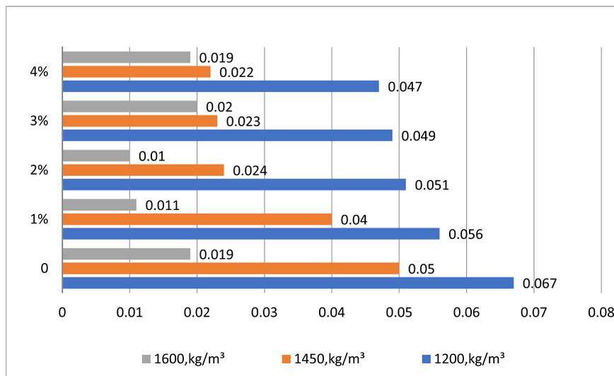
**Fig. 9.** The effect of Permeability with the addition of various percentage of fibers.
