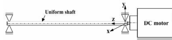
Figure.1. Schematic of DC motor driven flexible shaft
