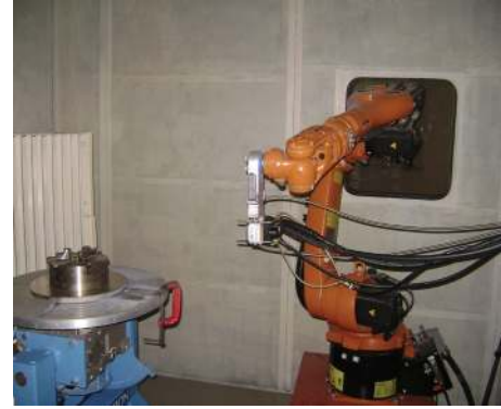
FIGURE 1: 80 kW atmospheric plasma spray system.
