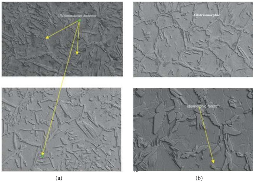
Figure 12: SEM photograph of PAW of duplex SS 2205 showing the various zones (a) Widmanstätten austenite and (b) allotriomorphic.
