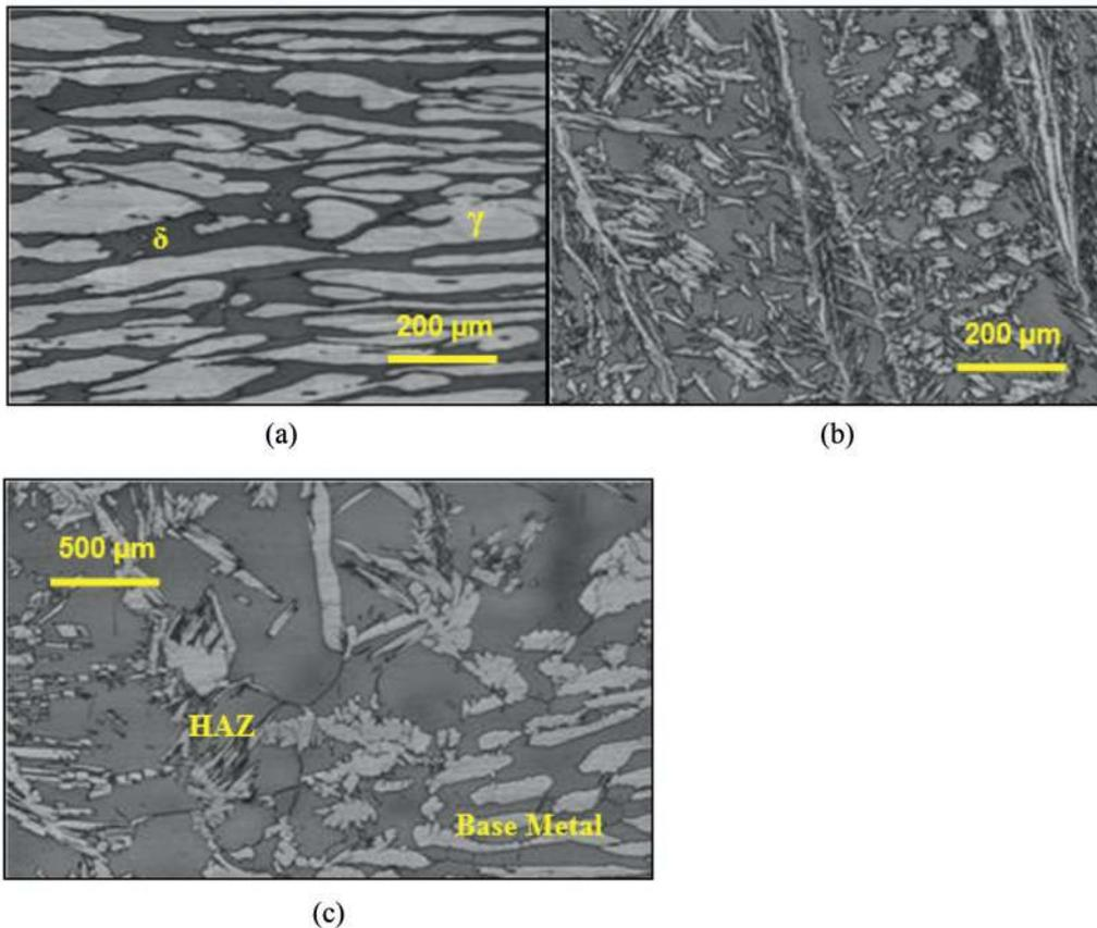
**Figure 9:** Microstructure of the (a) base metal: austenite is white and ferrite is dark (b) weld metal and (c) HAZ + base metal.
