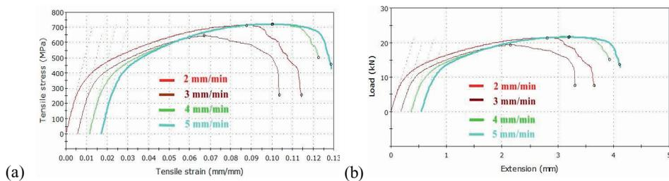
Fig.4. Graphs plotted between (a) Tensile Stress versus Tensile Strain (b) Load versus Extension
