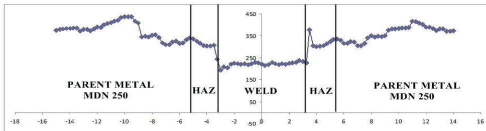
Fig.5. Hardness profile across the weld cross – section.
