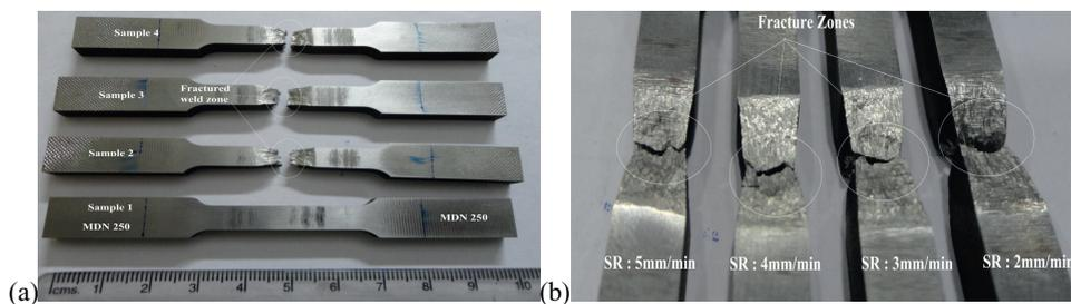
Fig. 3(a) Tensile Specimens tested at different strain rates (b) Fracture zones enlarged depicting nature of fracture
