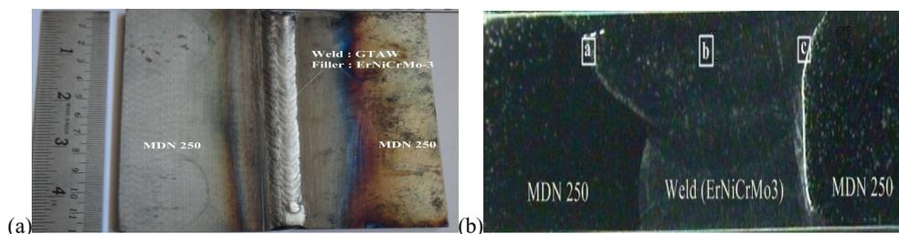
Fig. 1. Images of (a) As-welded sample. (b) Macrostructure of weld cross section.
