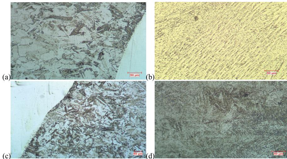
Fig. 2. Micrographs of (a) Interface on the left hand side (b) Weld region (c) Interface on the left hand side (d) Parent Metal of Maraging steel 250.
