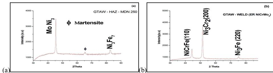
Fig. 6. XRD pattern of (a) HAZ of the Maraging steel (b) Weld Region.
