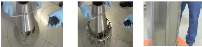
Fig.6. Experimental Investigation of Flow characteristics from left Slump Flow Test, in the centre U Box Test and at the right J-Ring Test
