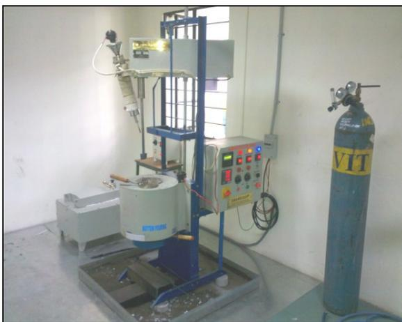
Fig.1 Fabrication of hybrid MMCs
