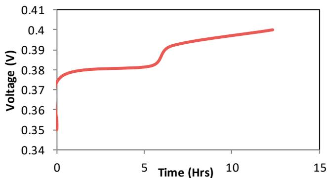
Fig. 6. OCP of EFC with 2X Conc. of MB
