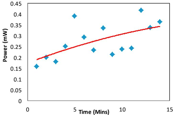
Fig. 13. Variation of MFC Power with time
