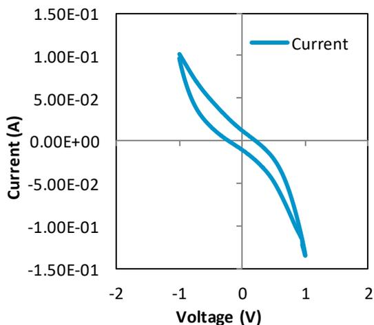
Fig. 7. Cyclic Voltammetry of EFC Before the Addition of Feed
