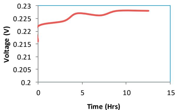
Fig. 2. OCP of MFC with Methylene Blue
