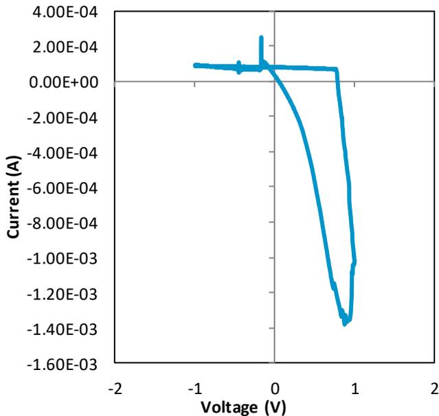
Fig. 11. Cyclic Voltammetry After the Addition of Feed and MB
