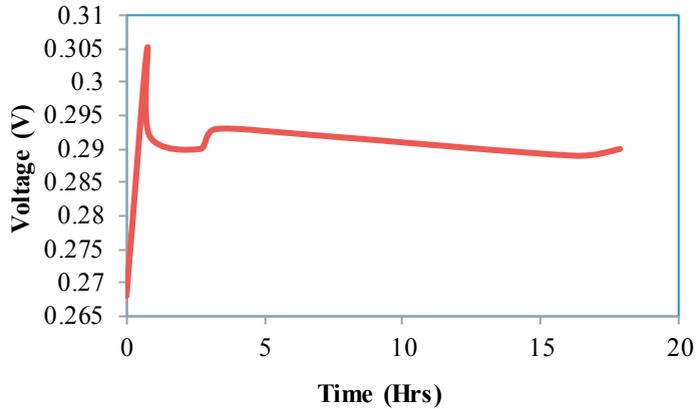
Fig. 3. OCP over time of the MFC with increased concentration of Methylene Blue.
