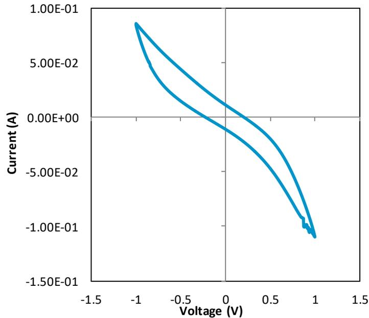
Fig. 10 Cyclic Voltammetry of MFC without Feed
