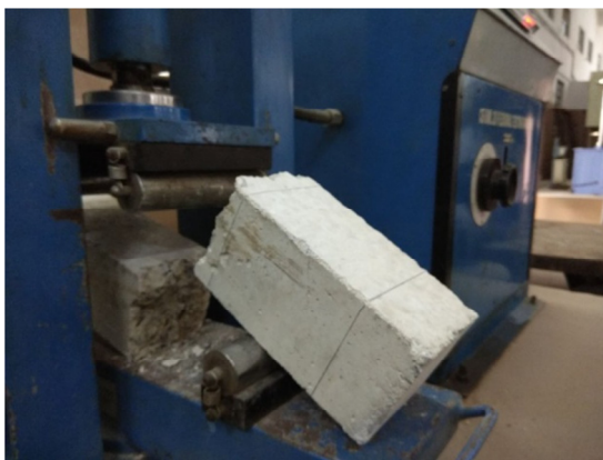
Fig6. Four- point loading setup
