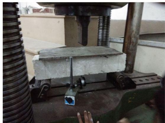
Fig7. UTM setup for load vs deflection analysis
