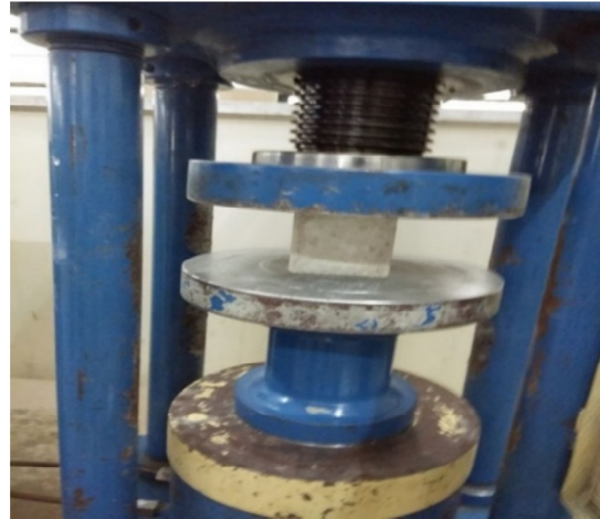
Fig1. Compressive strength test
