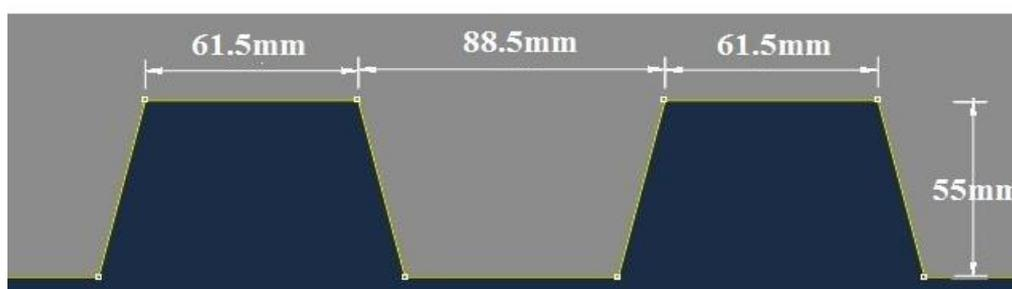
**Figure 2.** Dimensions of the profiled sheet
