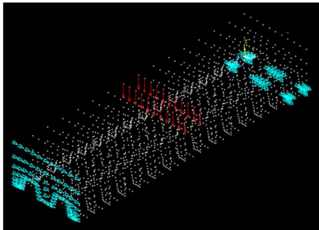
**Figure 4.** Plot of nodes with constraints and loading applied at nodes
