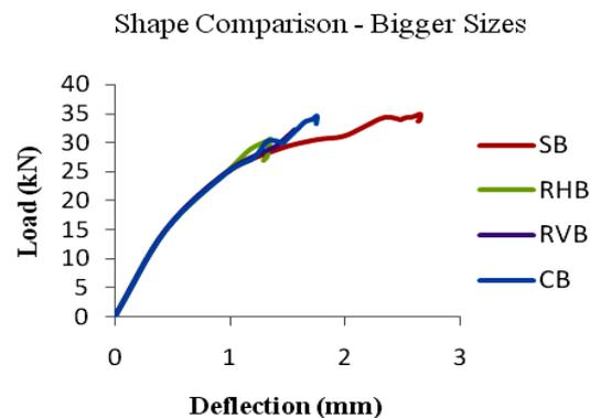
**Figure 13.** Comparison of load deflection curves for different shapes with bigger sizes
