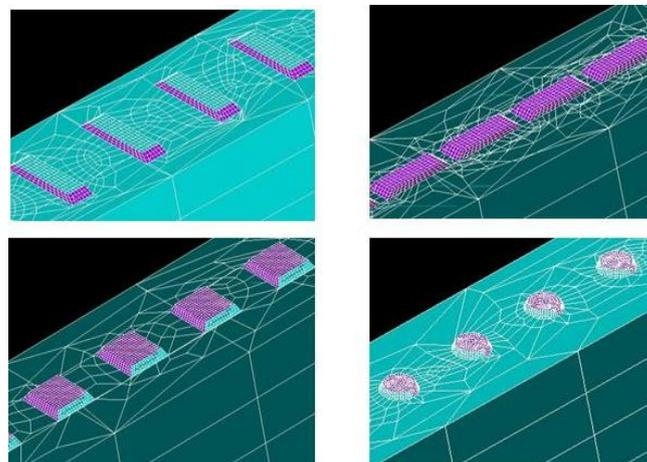
**Figure 3.** Meshed sheets clockwise from top left: with rectangular horizontal, rectangular vertical, circular and square embossments
