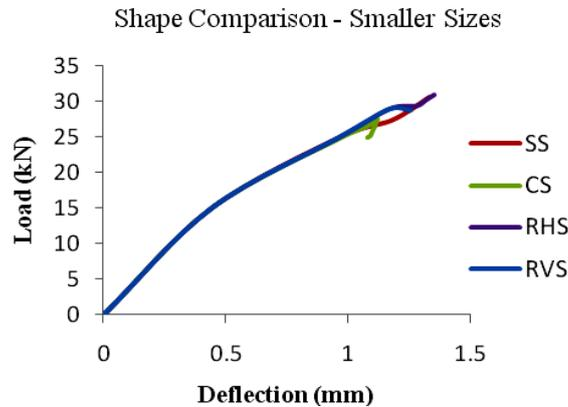
**Figure 12.** Comparison of load deflection curves for different shapes with smaller sizes
