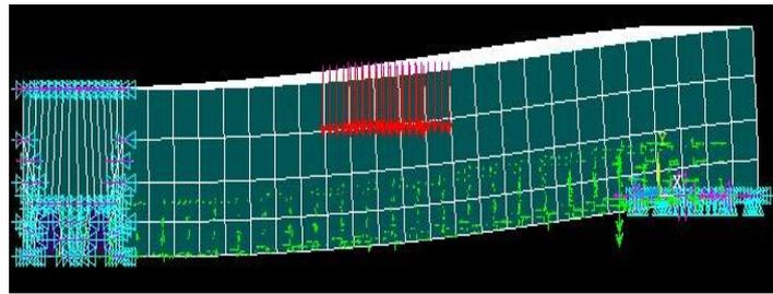
**Figure 6.** Deflected shape of composite slab after reaching ultimate load
