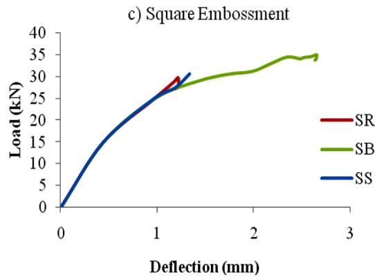
**Figure 9.** Comparison of load deflection curves for different sized embossments of square shape
