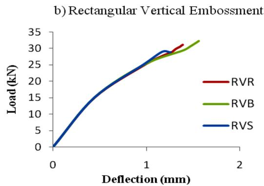
**Figure 8.** Comparison of load deflection curves for different sized embossments of rectangular shape vertically aligned
