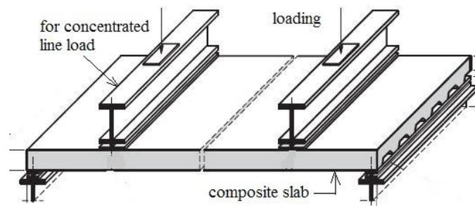
**Figure 1.** Loading of composite slab as per Eurocode 4
