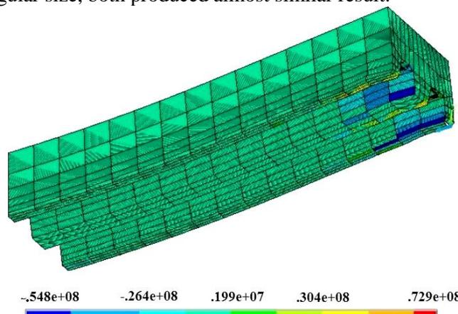
**Figure 14.** Longitudinal Shear Stress Plot for Slab with Square Bigger Type Embossment; values shown on scale in N/m<sup>2</sup>
