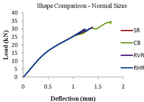
**Figure 11.** Comparison of load deflection curves for different shapes with normal sizes
