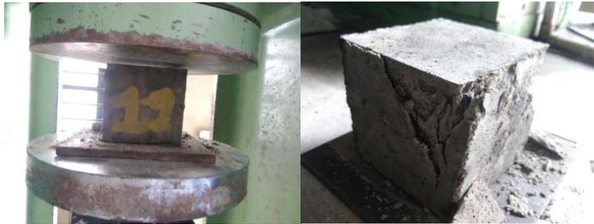
**Figure 1.** Testing and Failure Pattern of specimen
