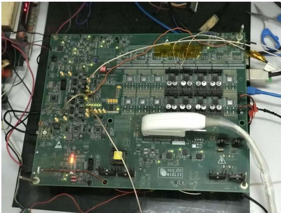
**FIGURE 16.** The custom ultrasound transceiver board.
