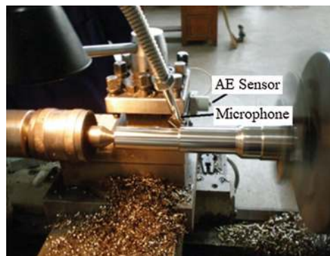
Figure 8: : Close-up view of sensors installation [66]
