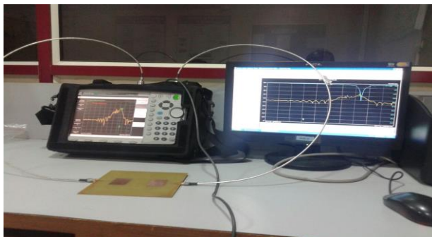
Figure 11 – Experimental set up of V.N.A.
