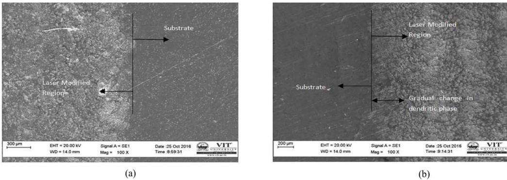
with coating shown in Figure 9(a) clearly dendritic phase, Zirconia and SiC are observed because of coating the heat absorbed is little when compared to sample3 laser peened without coating. The heat observed by sample3 composite of laser peened without coating is little high and it is reason for refinement of grains.
