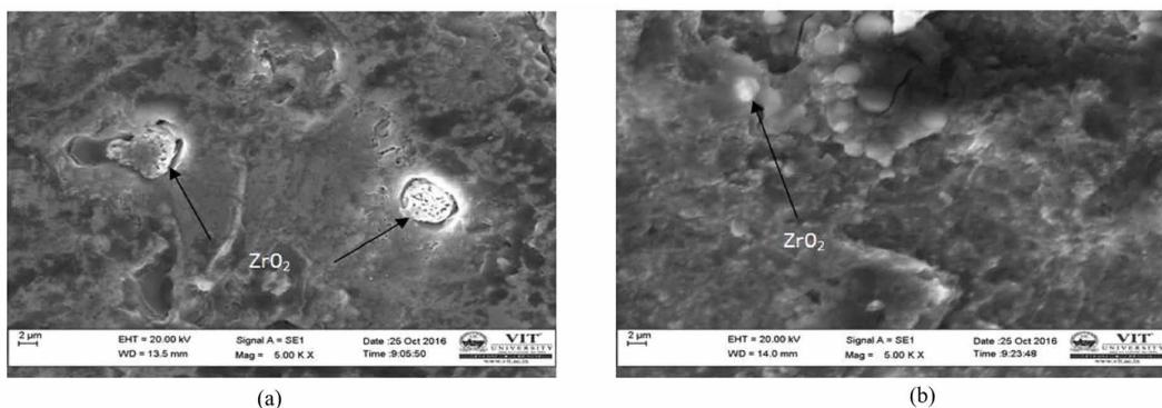
phase is clearly noticeable. But in Sample 3 laser-peened with coating shown in Figure 10(b) at same magnification the Zirconia particles can't be noticeable because the surface is modified with direct contact of laser beam pulse.
