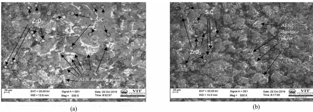
Figure 10. (a) SEM Sample 3 laser peened with coating at 5.0KX; (b) SEM Sample 3 laser peened without coating at 5.0KX
