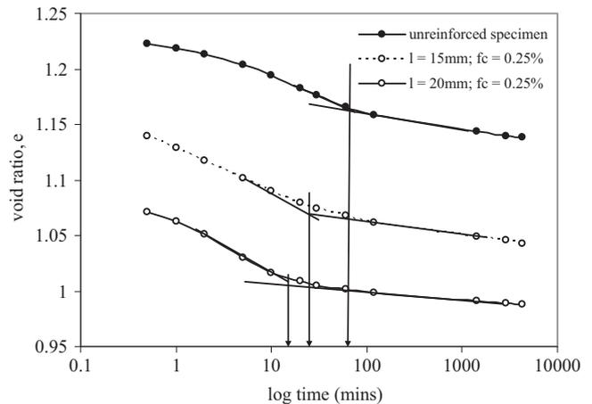
Fig. 7. Effect of fibre reinforcement on secondary consolidation.
