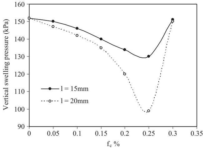
Fig. 6. Influence of fibre content on vertical swelling pressure.
