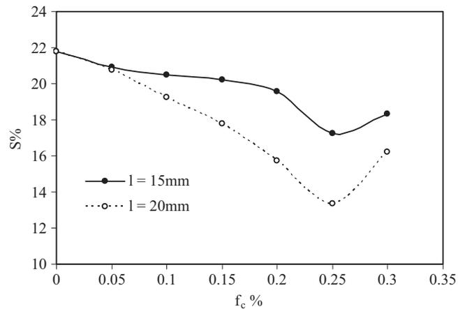
Fig. 5. Variation of swell potential with fibre content.
