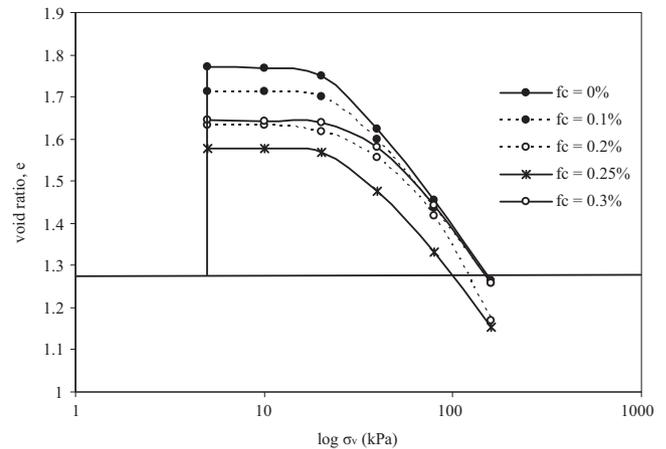
Fig. 4. e-log  $\sigma_v$  curves ( $l=20$  mm).
