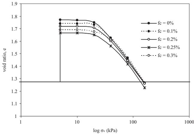
Fig. 3. e-log  $\sigma_v$  curves ( $l=15$  mm).
