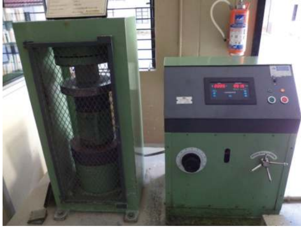
Fig. 3. Test set up for Compression testing machine
