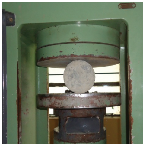
Fig. 7. Split tensile testing set up
