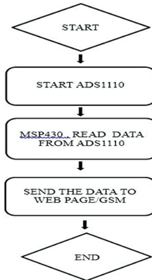
Figure 6 Flowchart of fuel level sensor mechanism
