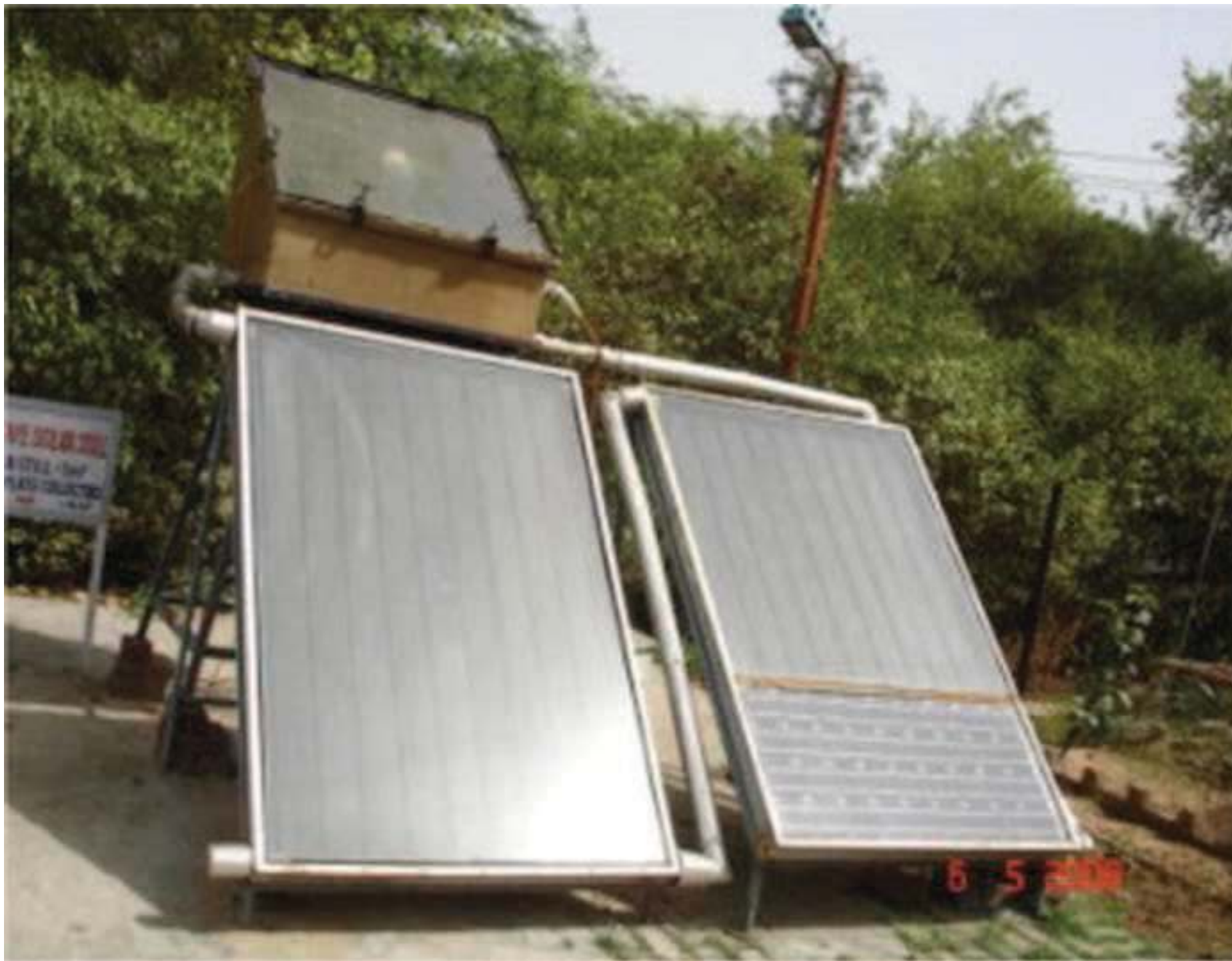
Fig. 6. Solar still integrated with photo-voltaic thermal (PVT). Click here to download high resolution image
