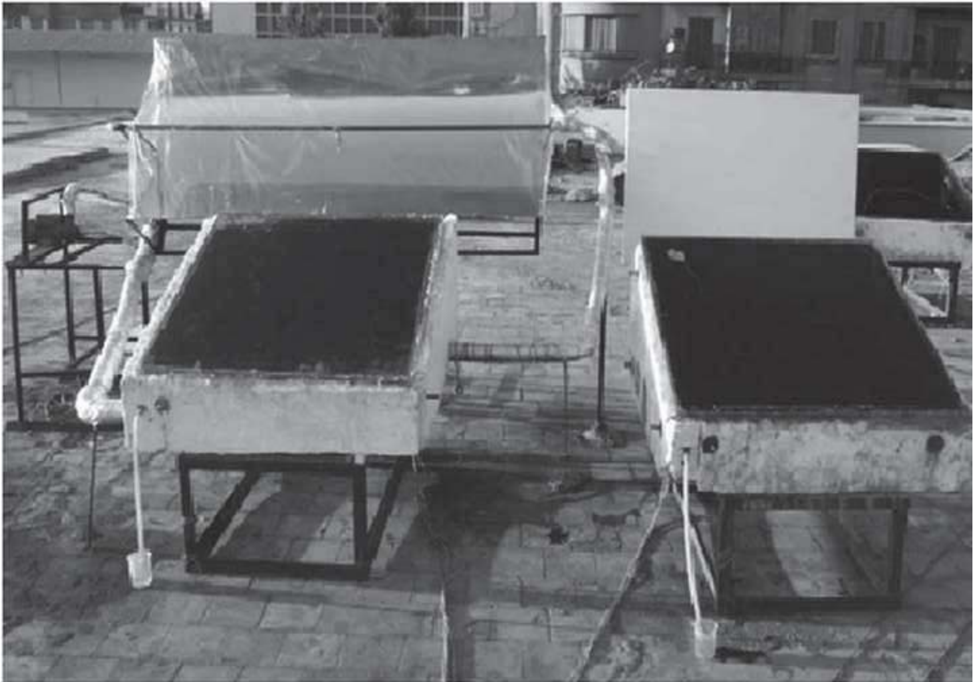
Fig. 6. Schematic of solar still integrated with concentrators. Click here to download high resolution image
