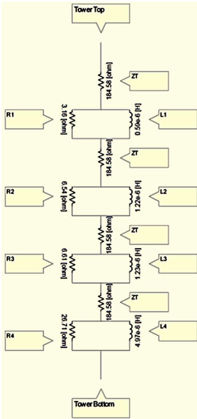
Fig. 5. Typical Tower Model created in PSCAD.
