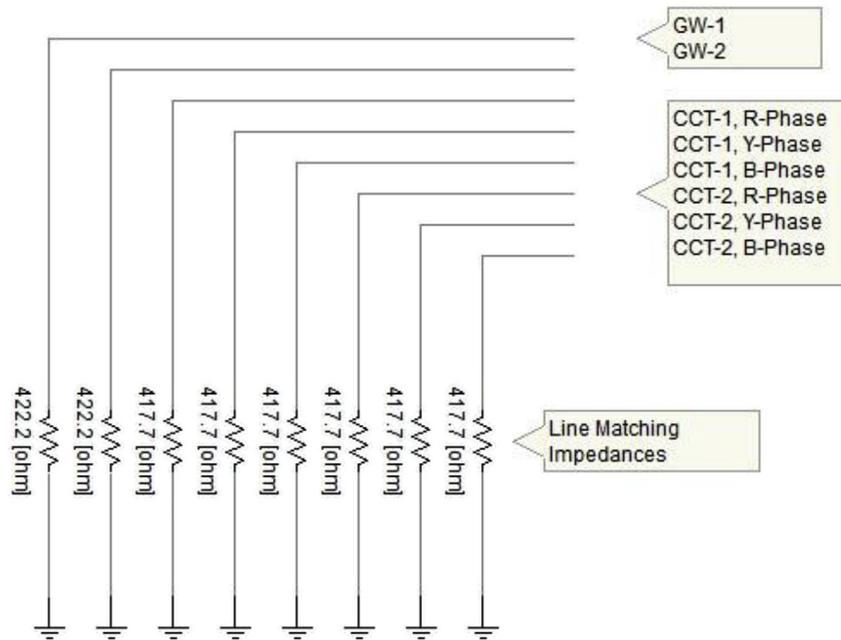
Fig. 10. Line Termination model created in PSCAD.
