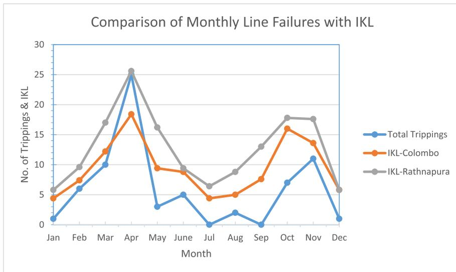
Fig. 1. Comparison of monthly line failures with IKL
