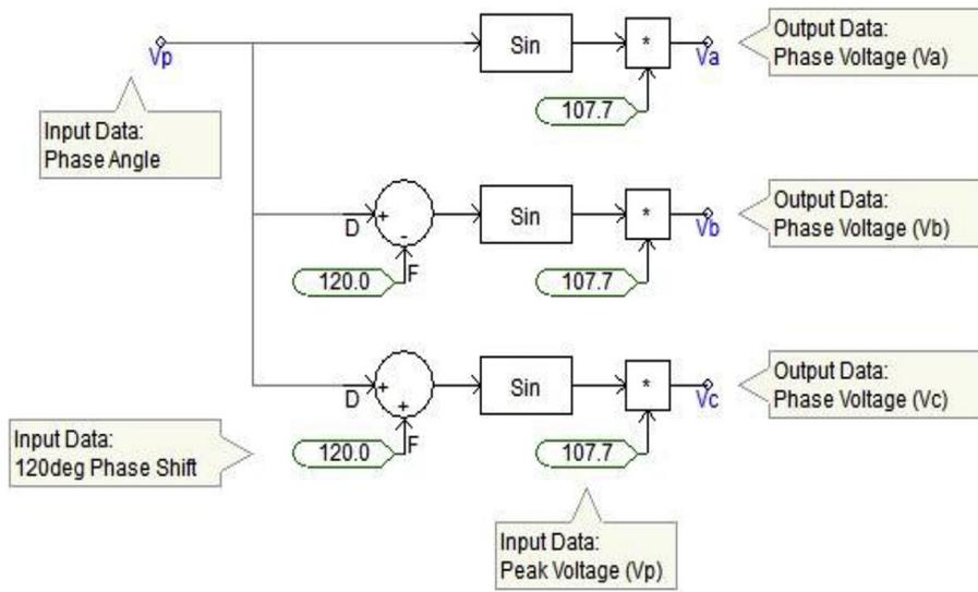
Fig. 9. Power frequency phase voltage generator model.
