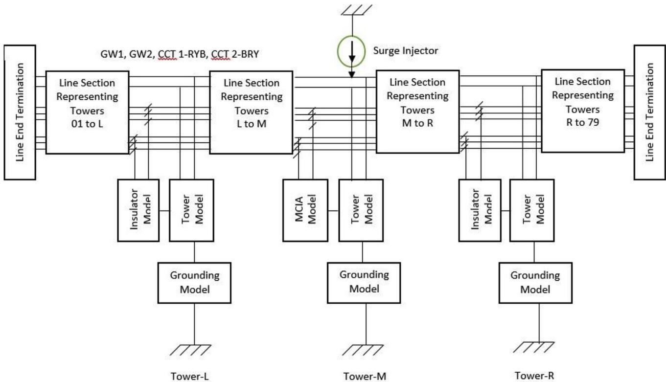
Fig. 3. Complete transmission line model for analysis.
