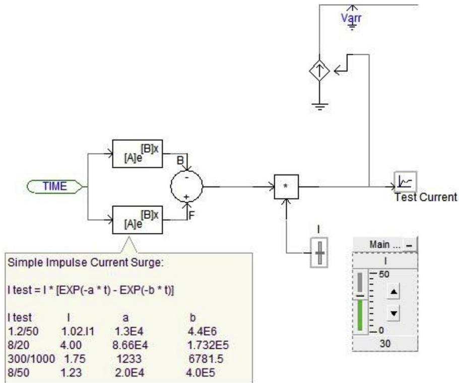
Fig. 16. Lightning Surge Generator Model created in PSCAD.
