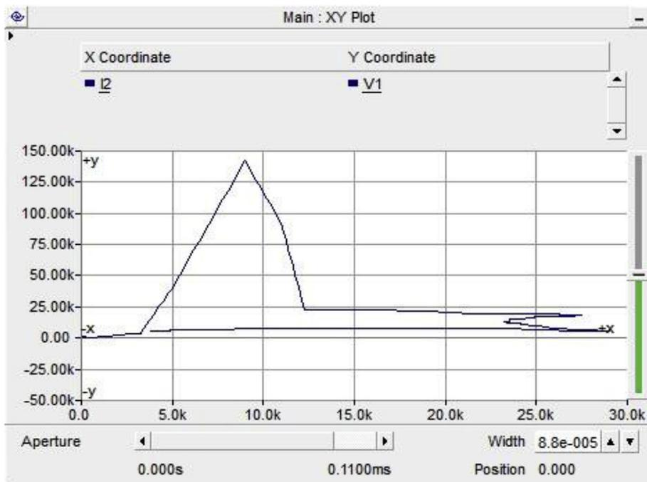
Fig. 13. MCIA model residual voltage variation with current.
