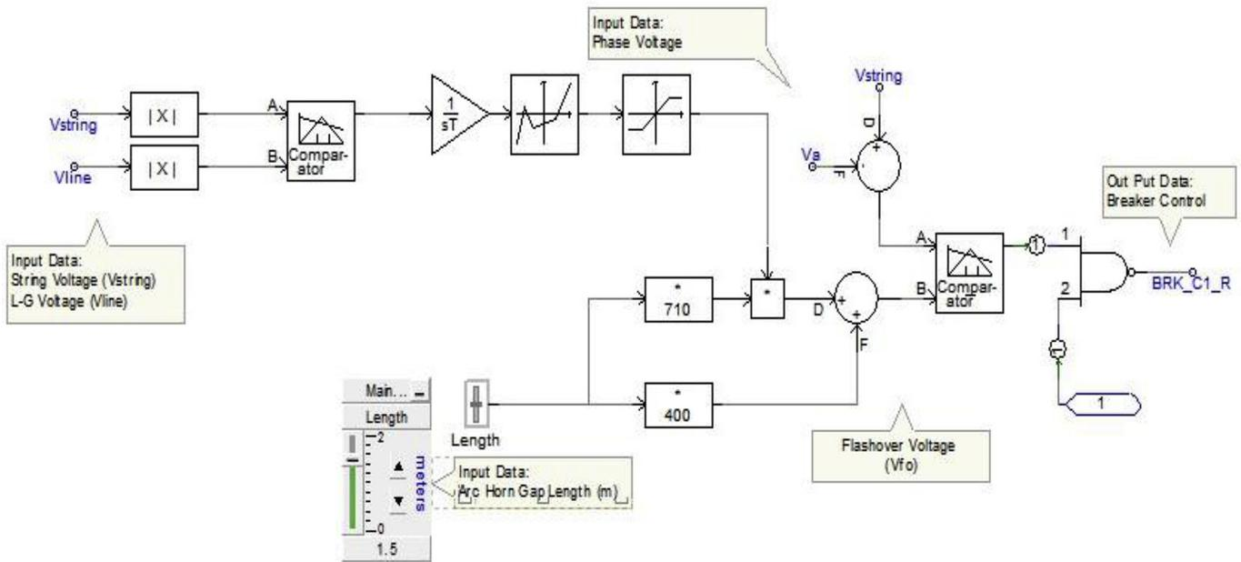
Fig. 8. Back-Flashover Control Module for conventional insulator string.
