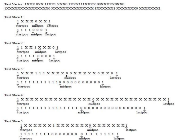
Fig.1: Illustration of filling the X-bits in the test cube with AERL-filling
