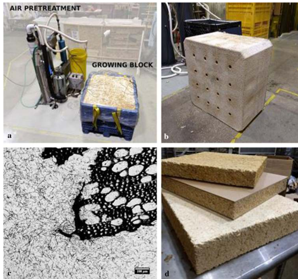
Fig. 44 a The bulk bin reactor system showing the air pretreatment system for air distribution and conditioning, and a bin incubation unit with a growing mycelium-lignocellulose composite block; b example of a bulk bin reactor system mycelium-lignocellulose block, after extraction from the bin incubation unit and prior to post-processing; c light micrograph of epoxy thin section of mycelium-wood composite, showing a two-dimensional section of the inter-particle hyphal matrix; d panels cut from a bulk bin reactor system mycelium-lignocellulose block during post-processing, showing examples of a sealed surface (top), an applied laminate (middle), and an unfinished surface (bottom)
