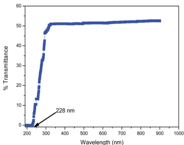
Fig. 12 The transmittance spectrum of the 2ADT crystal.
