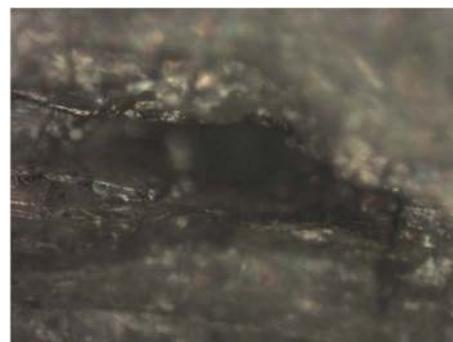
Fig. 17 Laser-induced damage on the 2ADT crystal surface.
