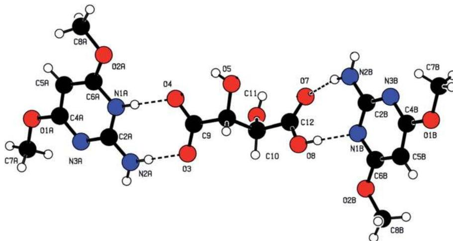
Fig. 7 The three-dimensional molecular structure of the 2ADT salt. The N–H...O and O–H...N contacts are shown as thin dashed lines.
