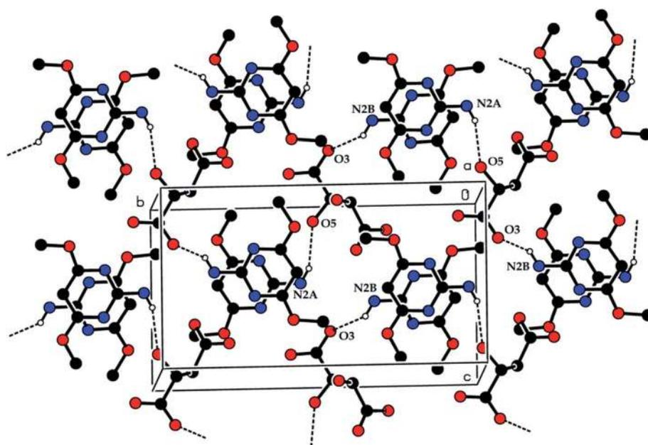
Fig. 8 The N2A-H2A1...O5<sup>i</sup> and N2B-H2B2...O3<sup>ii</sup> intermolecular hydrogen bonds. [Symmetry code: (i)  $x, y, 1 + z$  and (ii)  $x, y, -1 + z$ ].
