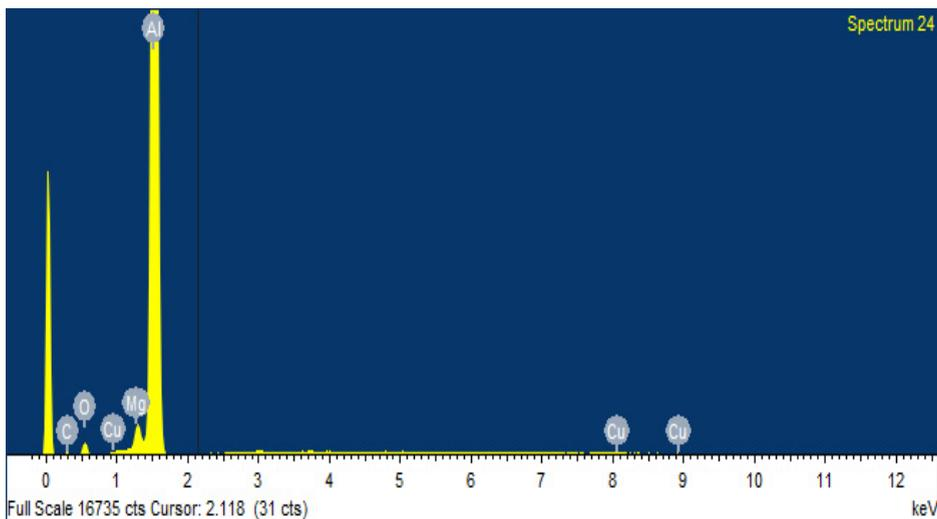
Figure 3: EDAX microstructure of Al6061 + 5% by wt egg shell
