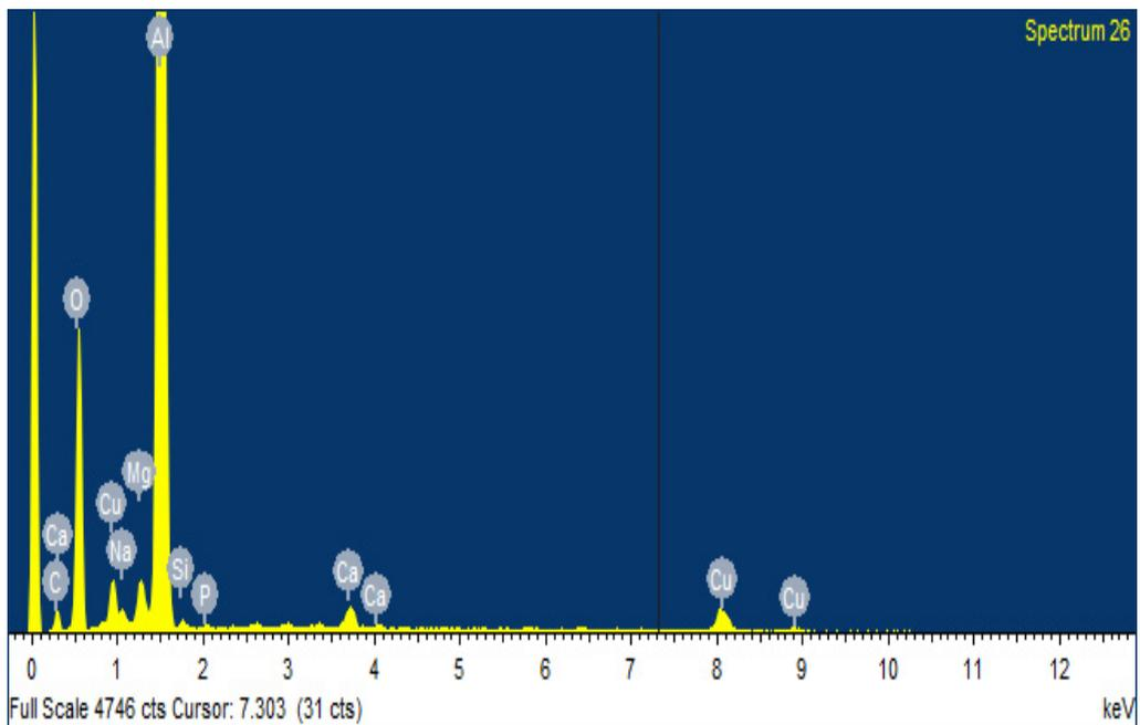
Figure 5: EDAX of the Al6061 + 10% by wt egg shell
