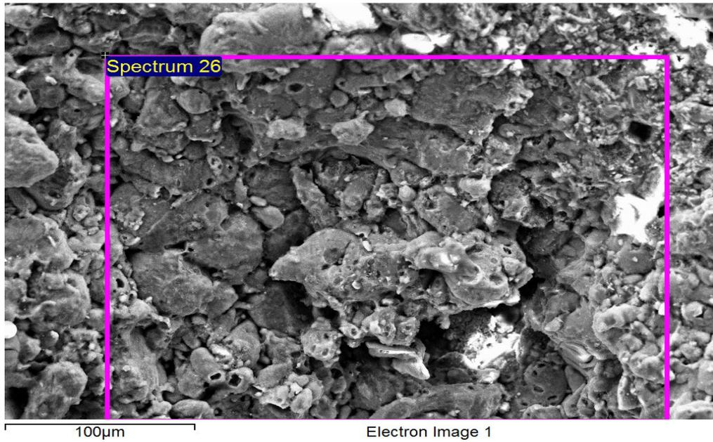
Figure 4: SEM image of Al6061 + 10% by wt egg shell
