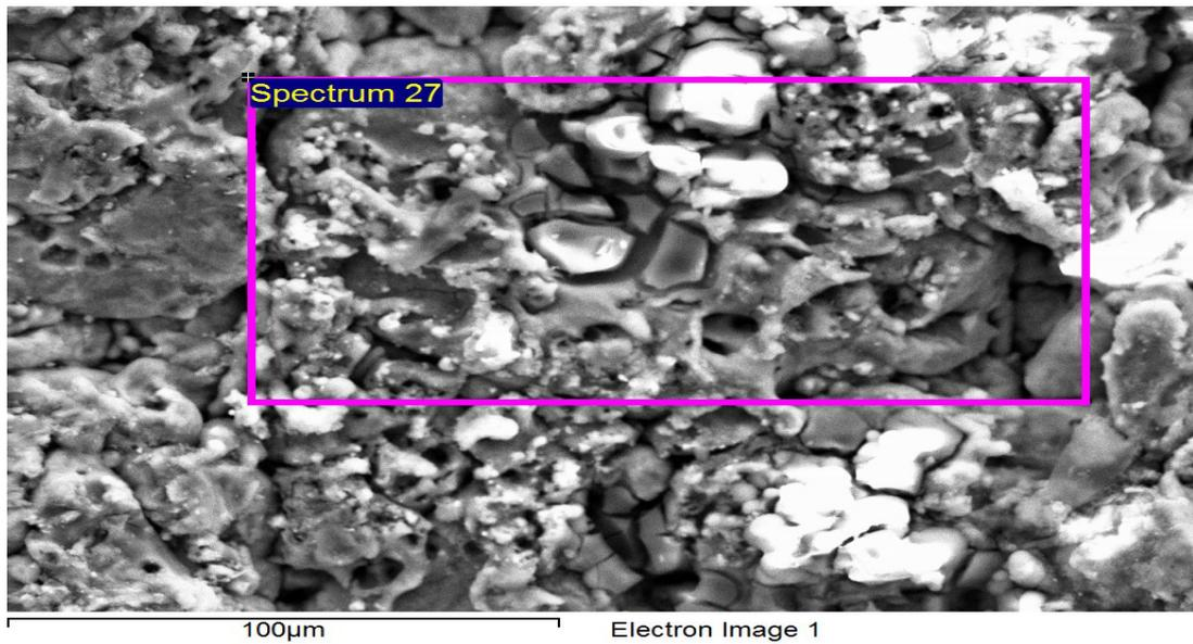
Figure 6: SEM image of Al6061 + 15% egg shell
