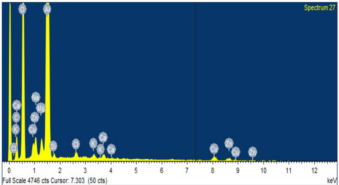
Figure 7: EDAX microstructures of Al6061 + 15% egg shell.
