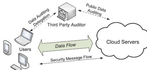
Fig. 5. The architecture of cloud data storage service [3]
