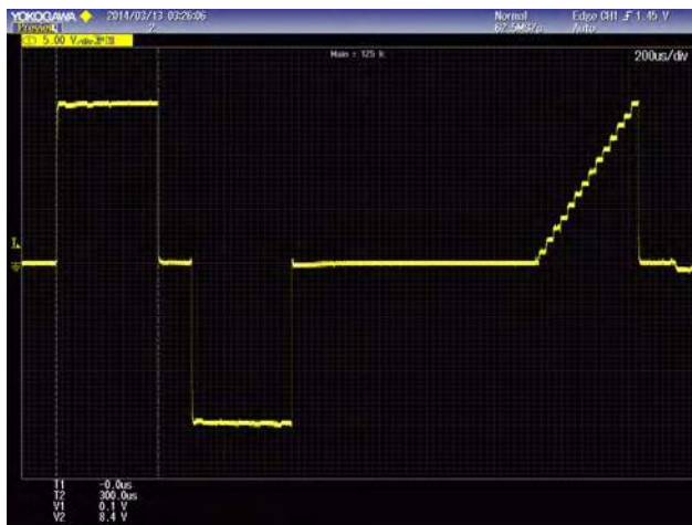
Figure 5 Generated waveform on a 1k \Omega resistive load.
