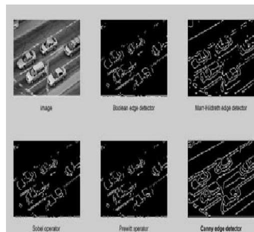
Fig 2: Different edge detection techniques
