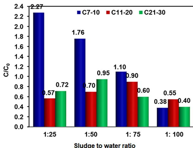
Fig. 4. Effect of sludge to water ratio on PHC degradation using sono-Fenton process (Sludge/water ratio = 1:100,  $\text{H}_2\text{O}_2/\text{Fe}^{2+}$  weight ratio = 10:1, ultrasonic power = 100, contact time = 10 min).
