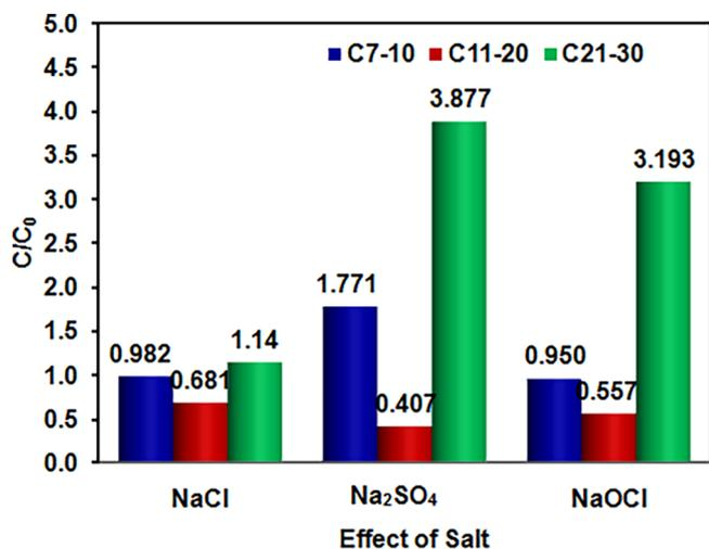
Fig. 9. Effect of PHC degradation in the presence of different salts (pH = 3, sludge/water ratio = 1:100, ultrasonic power = 100 W, H<sub>2</sub>O<sub>2</sub>/Fe<sup>2+</sup> weight ratio = 10:1, treatment time = 10 min).
