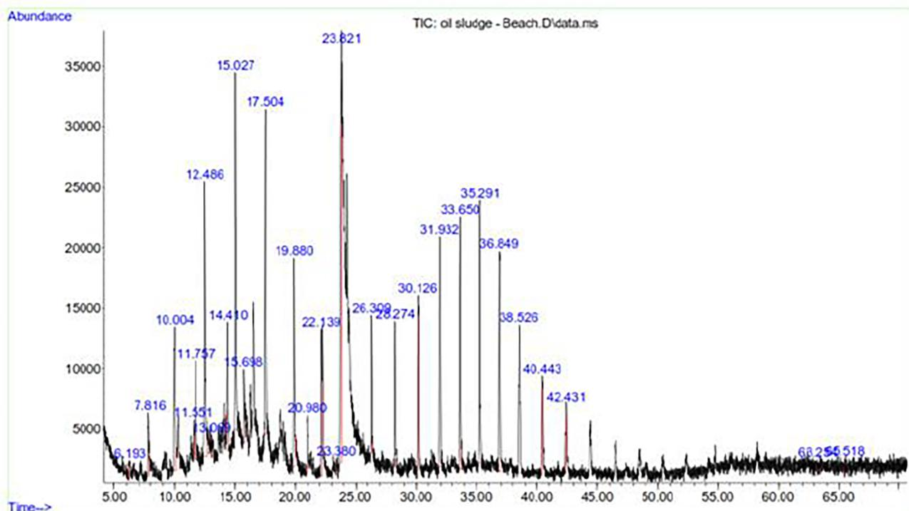
Fig. 1. Gas chromatograph of sludge sample collected 10 days after the oil spill.
