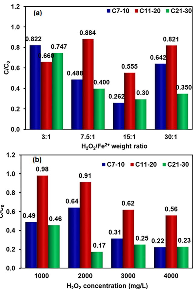
Fig. 7. (a) Effect of  $\text{H}_2\text{O}_2/\text{Fe}^{2+}$  weight ratio on PHC degradation in oil spill sludge (b) Effect of varying  $\text{H}_2\text{O}_2$  concentration with the fixed  $\text{H}_2\text{O}_2/\text{Fe}^{2+}$  weight ratio of 10:1 (pH = 3, sludge/water ratio = 1:100, ultrasonic amplitude 40%, contact time = 10 min).
