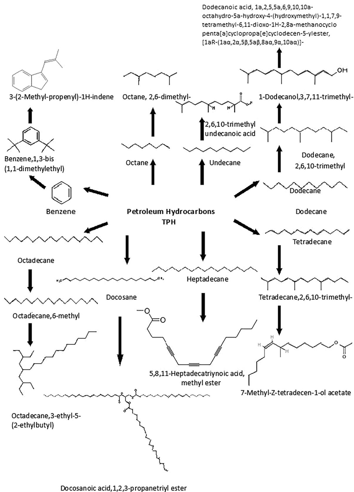
Fig. 10. Proposed mechanism for Fenton assisted ultrasound treatment.
