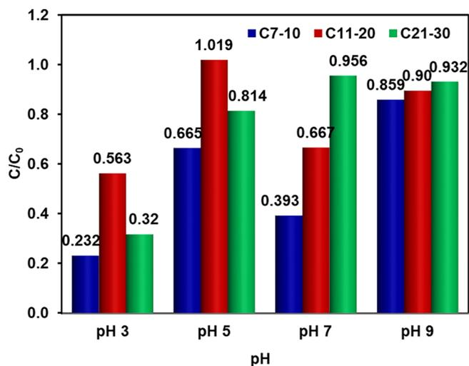
Fig. 5. Effect of pH on PHC degradation using sono-Fenton process (Sludge/water ratio = 1:100,  $\text{H}_2\text{O}_2/\text{Fe}^{2+}$  weight ratio = 10:1, ultrasonic power = 100, contact time = 10 min).
