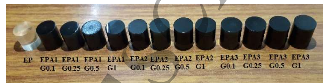
Figure 2 Prepared neat epoxy and Al 2 O 3 and GnP reinforced epoxy nanocomposites samples for hardness test.
