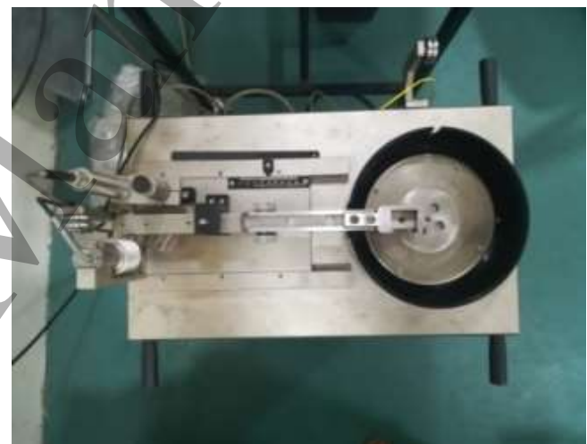
Figure 3 Pin on disc test setup.
